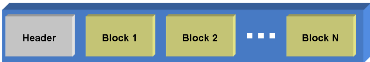
Figure 1-2 : Inside a Load Image
