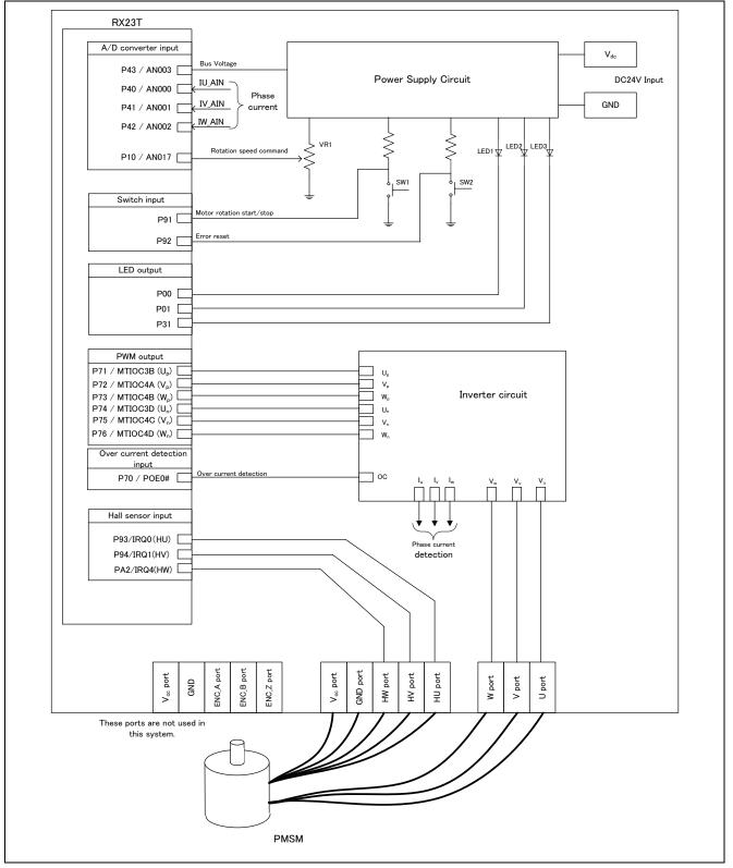
Figure 2-1 Hardware Configuration Diagram
