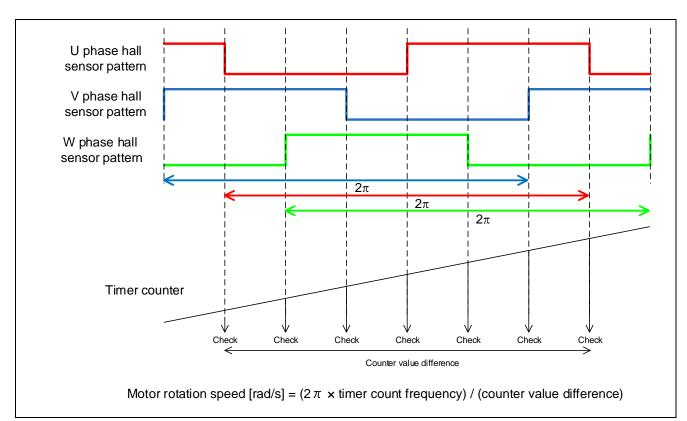
Figure 3-1 Motor Rotation Speed Calculation Method
