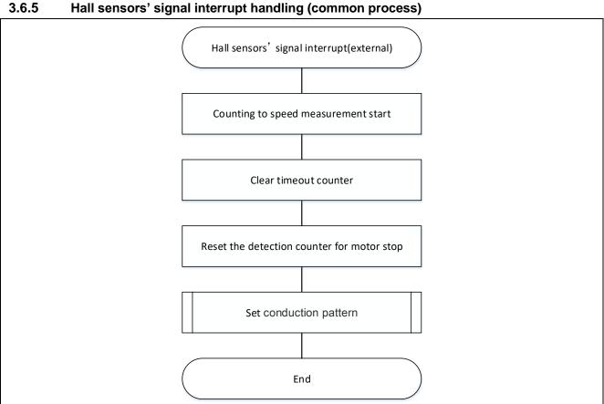
Figure 3-11 Hall sensors' signal Interrupt Handling (common process)
