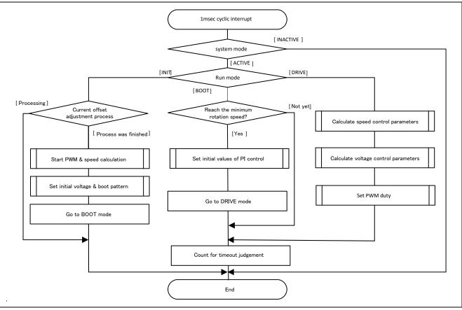
Figure 3-9 1 [ms] Interrupt Handling
