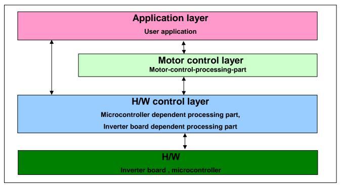
Figure 2-2 Module Configuration of the Sample Programs
