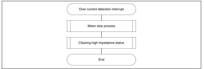
Figure 3-10 Over Current Detection Interrupt Handling
