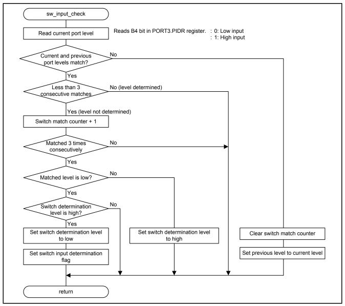
Figure 5.10 Switch Input Determination
