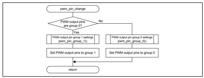
Figure 5.7 PWM Output Pin Switching
