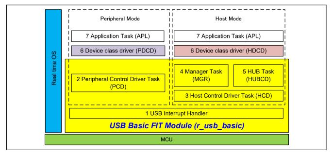
Figure 1-2 USB Software Configuration of USB-BASIC-FW (FreeRTOS, uITRON)
