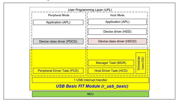
Figure 1-1 USB Software Configuration of USB-BASIC-FW (Non-OS)
