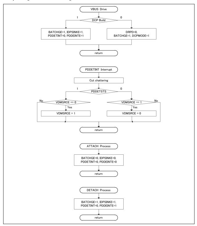
Figure 3-1 HBC processing flow
