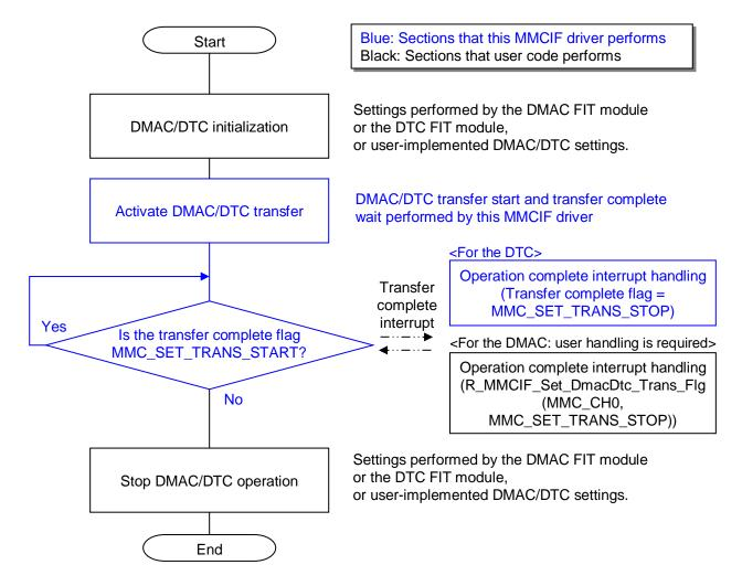
Figure 1.5 Processing for DMAC/DTC Transfer Setup
