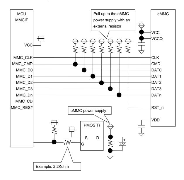
The n in DATn indicates lines 4 to 7. Connect a pull-up resistor each line in DAT4 to DAT7. The figures shows the case where the same 2.7 to 3.6V power supply is supplied to both the VCC and VCCQ eMMC pins
