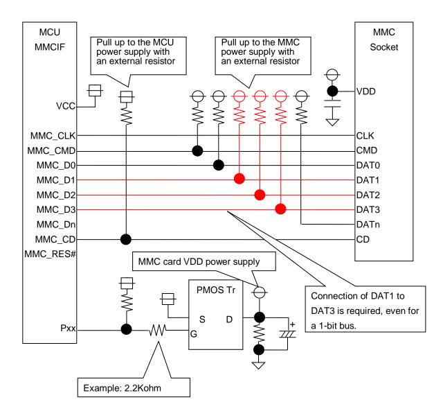
The n in DATn indicates lines 4 to 7. Connect a pull-up resistor each line in DAT4 to DAT7.
