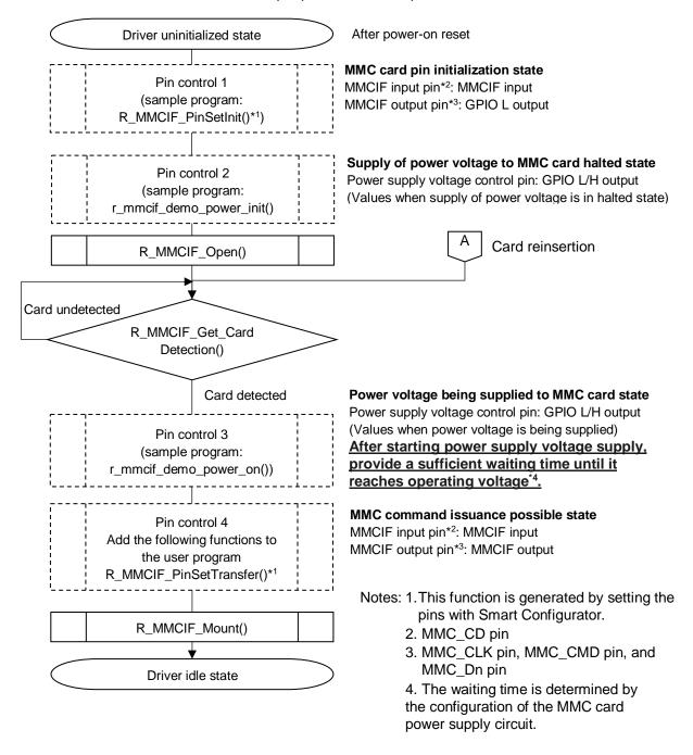
Figure 4.1 MMC card Insertion and Power-On Timing
