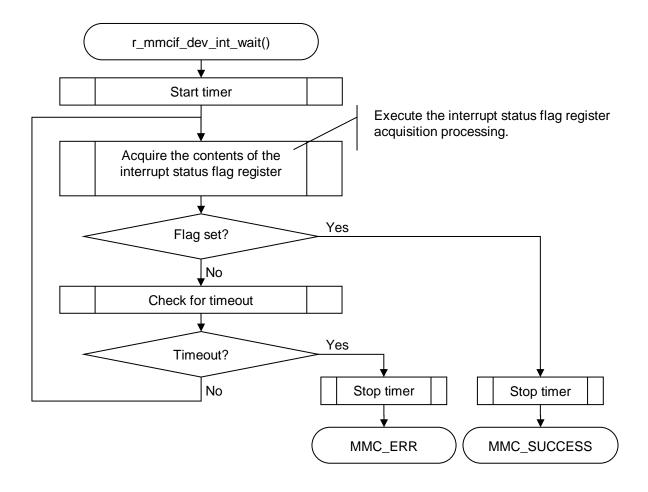
Figure 1.3 MMC Protocol Status Verification Using Software Poling
