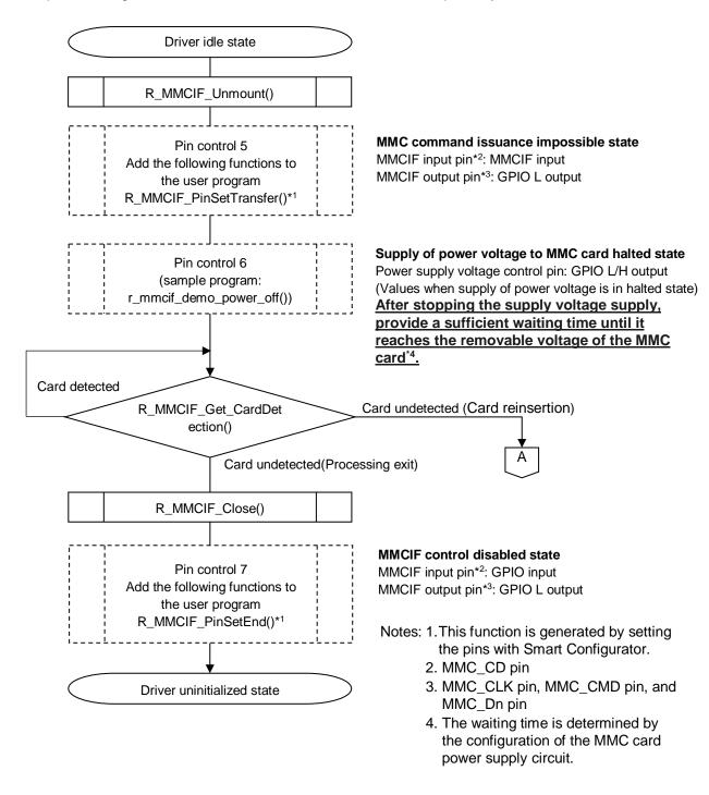
Figure 4.2 MMC card Removal and Power-Off Timing
