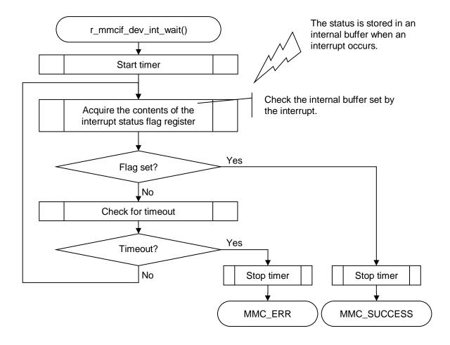
Figure 1.4 MMC Protocol Status Verification Using Interrupts
