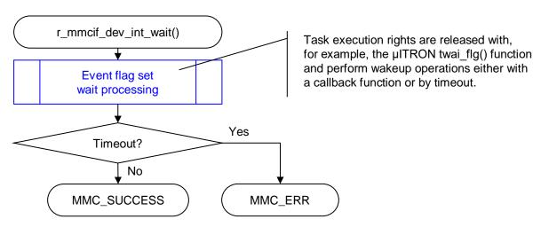
Figure 6.2 MMC Protocol Status Verification Example Using Operating System Wait Task Processing
