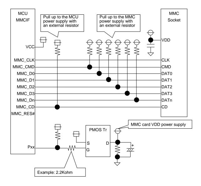
The n in DATn indicates lines 4 to 7. Connect a pull-up resistor each line in DAT4 to DAT7.
