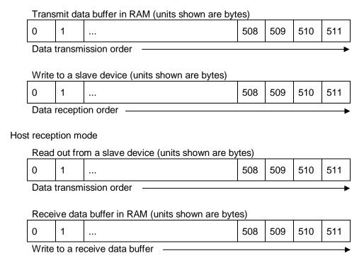
Figure 1.2 Transmission Data Storage
