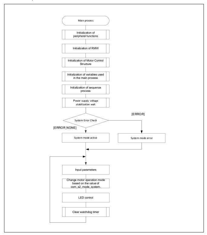
Figure 3-27 Main Process Flowchart
