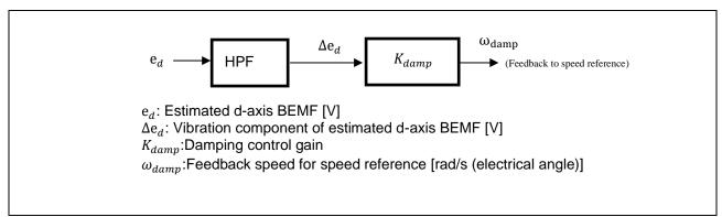
Figure 3-22 Block diagram of the open loop damping control
