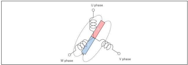
Figure 3-15 Relationship between rotor position and each phase
