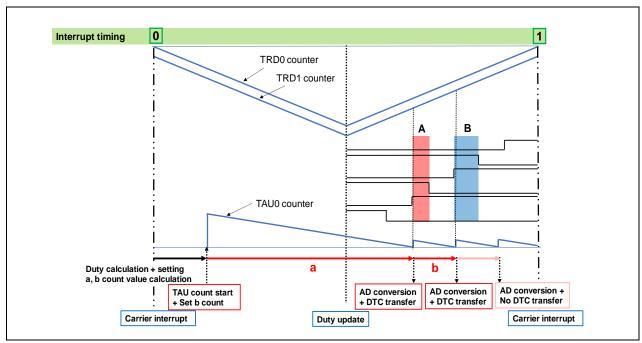
Figure 3-11 Timing of A/D Conversion
