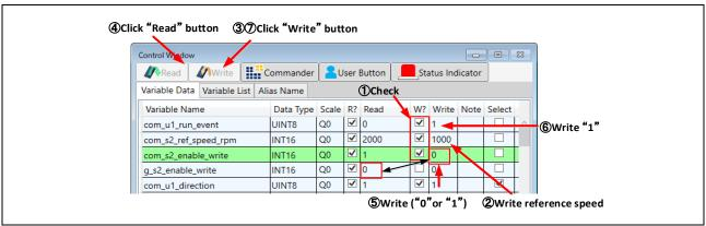
Figure 4-2 Procedure - Driving the motor
