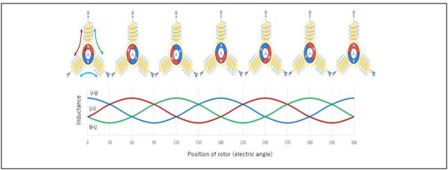
Figure 3-14 Changes in inductance according to rotor position
