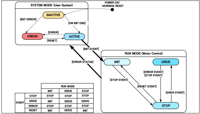
Figure 3-5 State Transition Diagram
