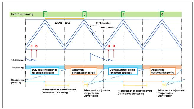
Figure 3-13 Periodic duty adjustment and compensation
