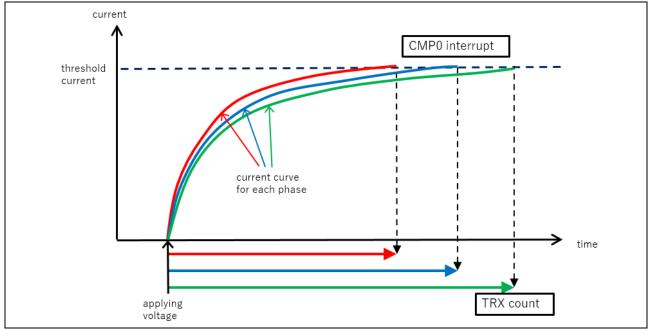
Figure 3-17 Current detection time differential among the 3 Phases
