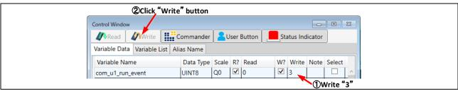
Figure 4-4 Procedure - Error cancel operation
