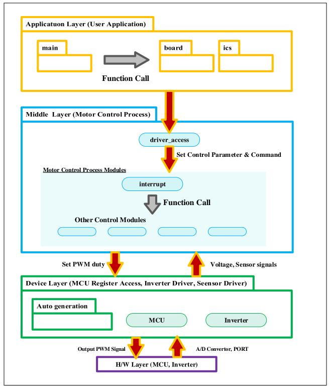
Figure 2-2 Module Configuration of the Sample Programs
