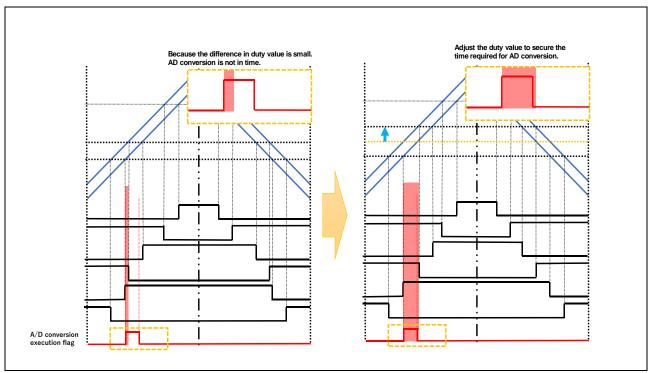
Figure 3-12 Duty adjustment (example)
