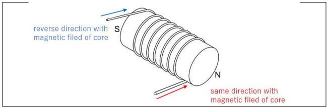
Figure 3-19 Example of magnetic pole wound with coil
