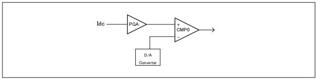
Figure 3-2 Overcurrent detection by CMP0
