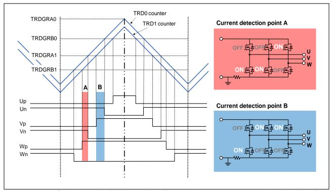
Figure 3-10 Complementally PWM waveform (For example, duty magnitude relation W > V > U).
