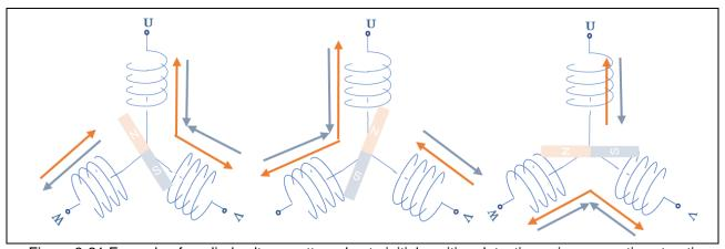
Figure 3-21 Example of applied voltage pattern due to initial position detection using magnetic saturation
