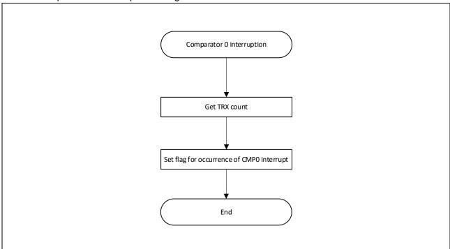
Figure 3-32 Comparator 0 interrupt handling
