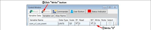
Figure 4-3 Procedure - Stop the motor
