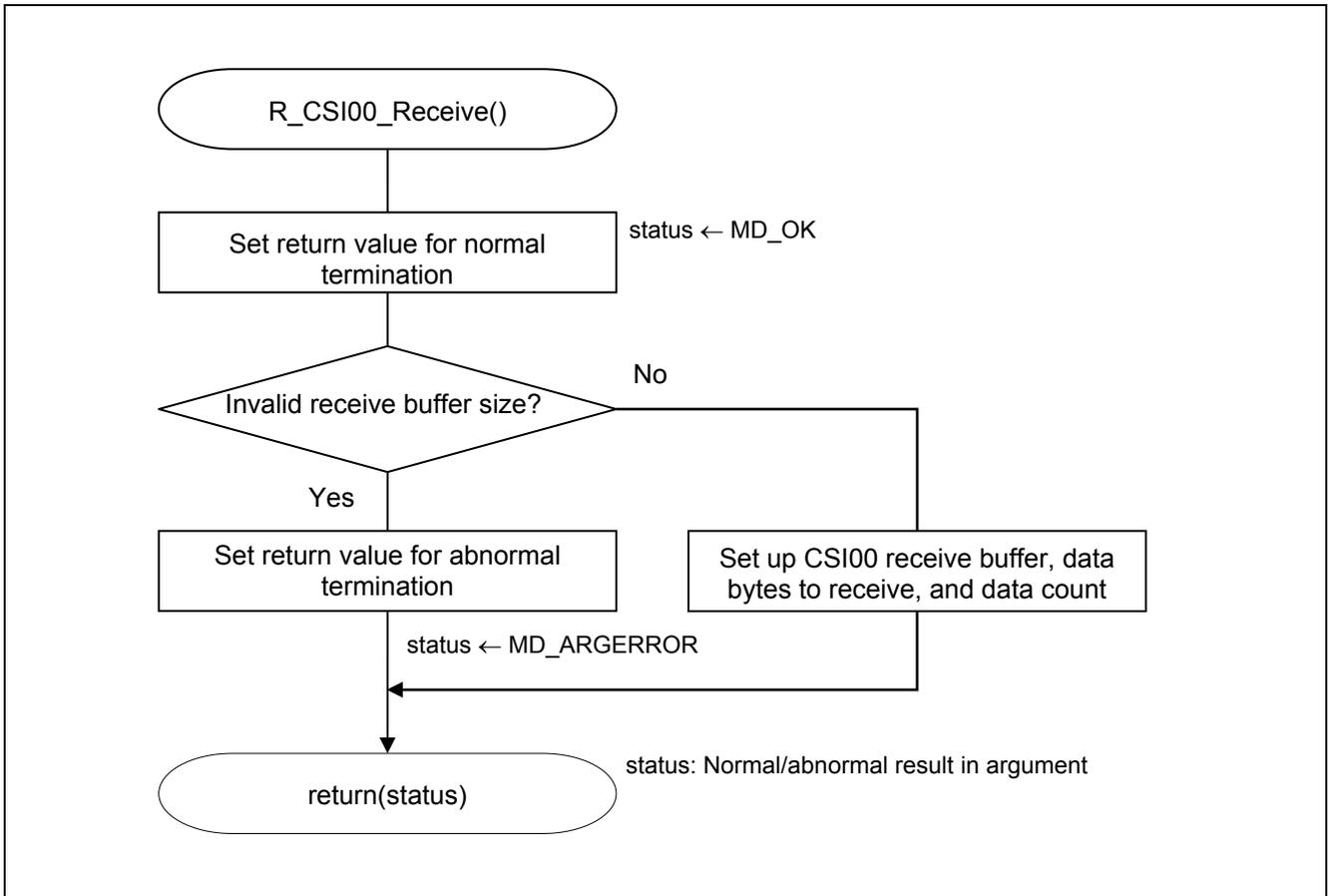
**Figure 5.16 Setting up the CSI00 Receive Buffer**
