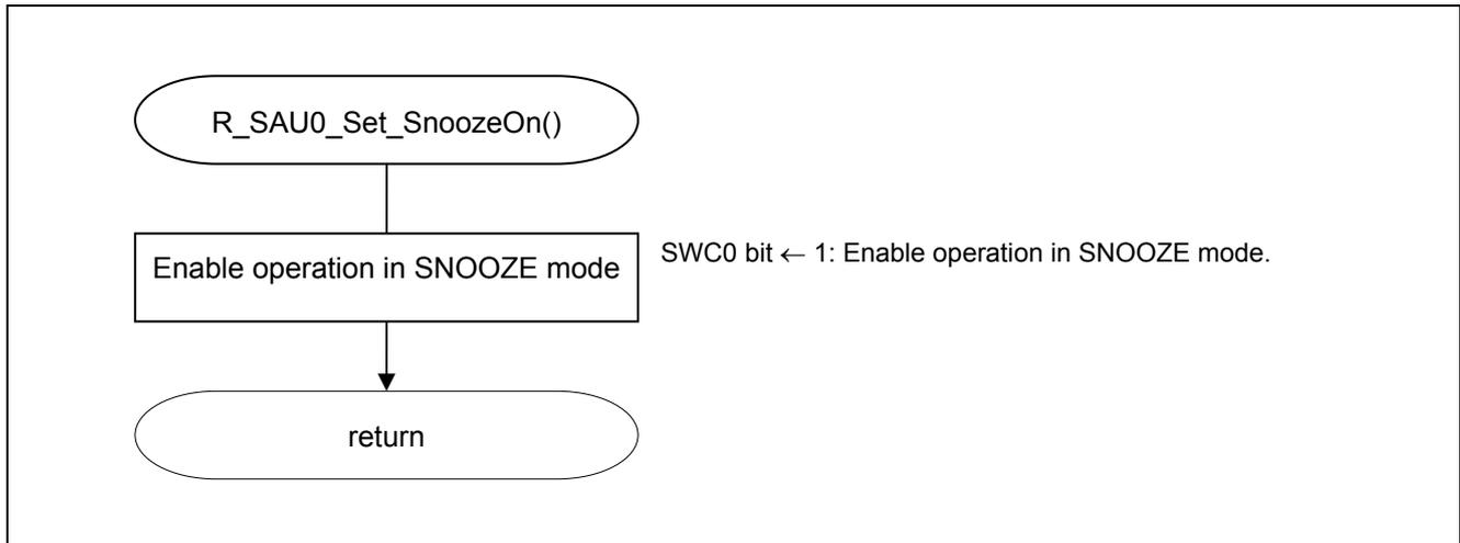
Figure 5.12 Enabling CSI00 in SNOOZE Mode
