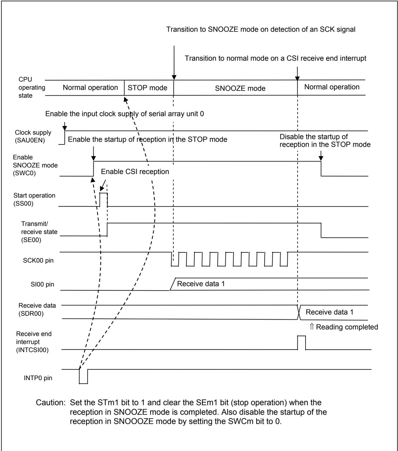
Figure 1.3 Timing Chart of SNOOZE Mode
