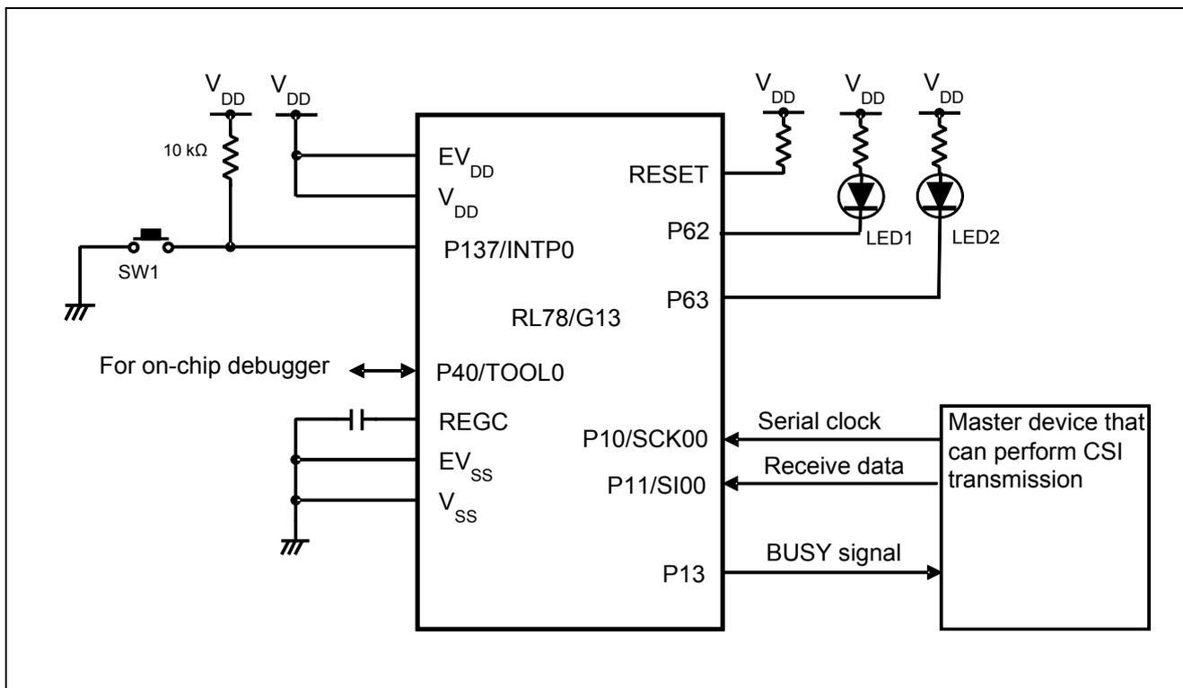
**Figure 4.1 Hardware Configuration**
