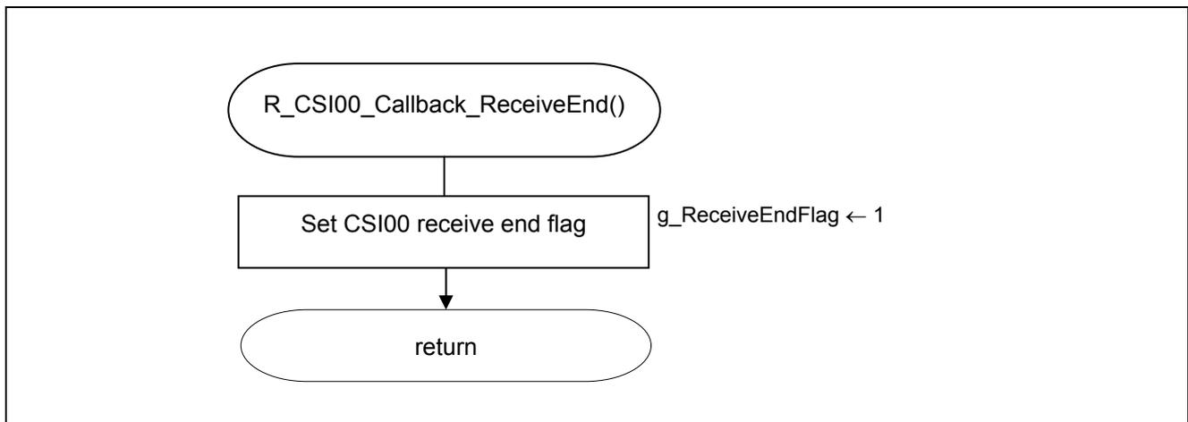
**Figure 5.18** Callback Function for SI00 Communication End Interrupts
