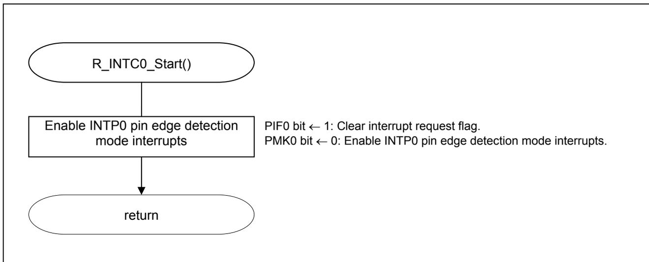
Figure 5.21 Starting INTP0 Operation
