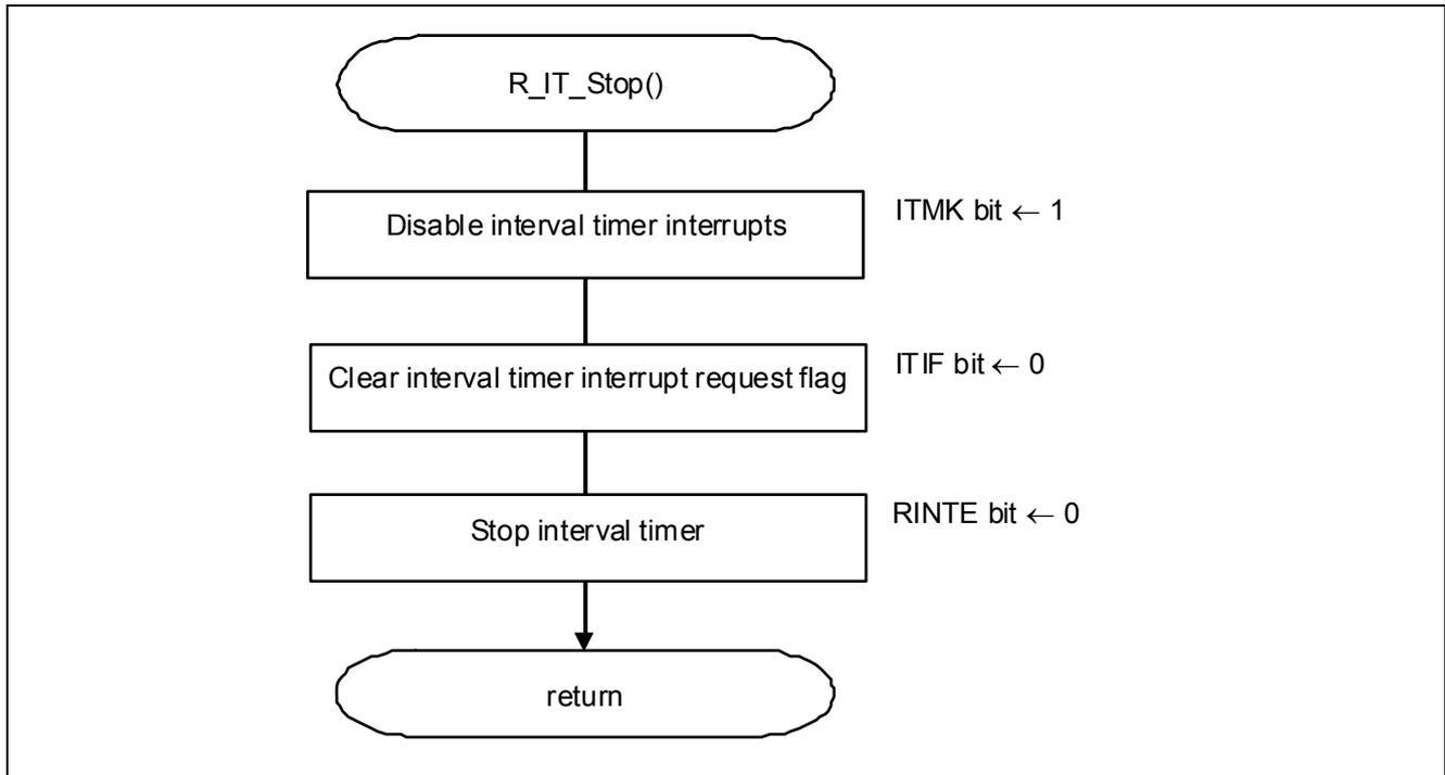
Figure 5.25 Stopping Interval Timer
