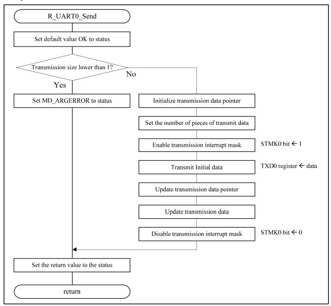
Figure 5.17 UART0 data transmission function
