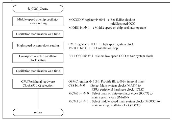
Figure 5.7 CPU clock initialization function
