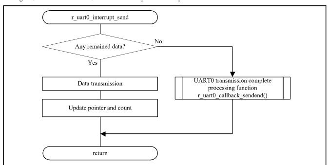
Figure 5.21 UART0 transmission complete interrupt function
