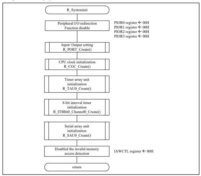
Figure 5.5 Peripheral function initialization function
