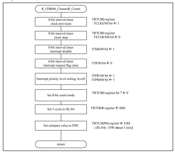
Figure 5.10 8-bit interval timer initialization function
