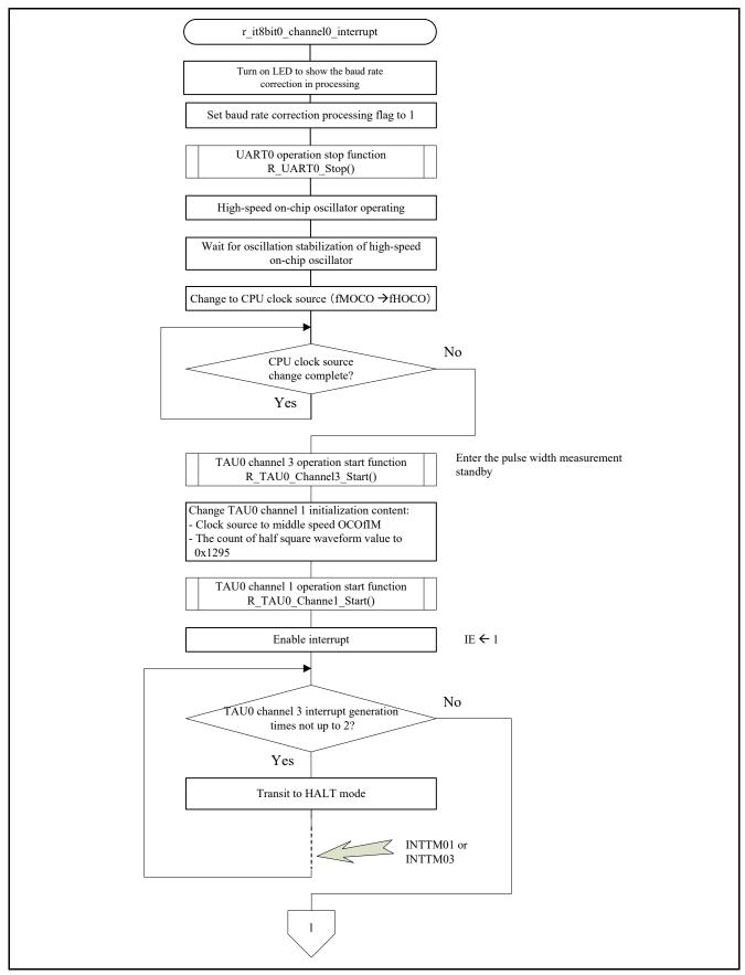
Figure 5.22 8-bit interval timer interrupt function (1/2)
