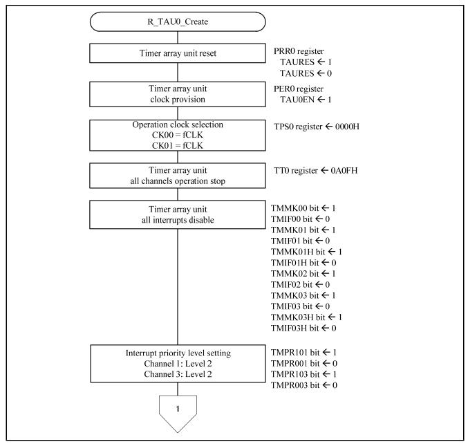
Figure 5.8 Timer array unit initialization(1/2)
