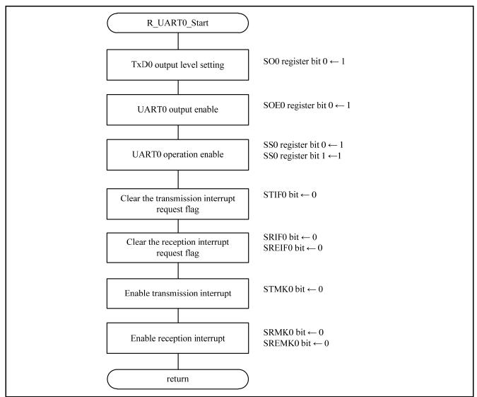
Figure 5.16 UART0 operation start function
