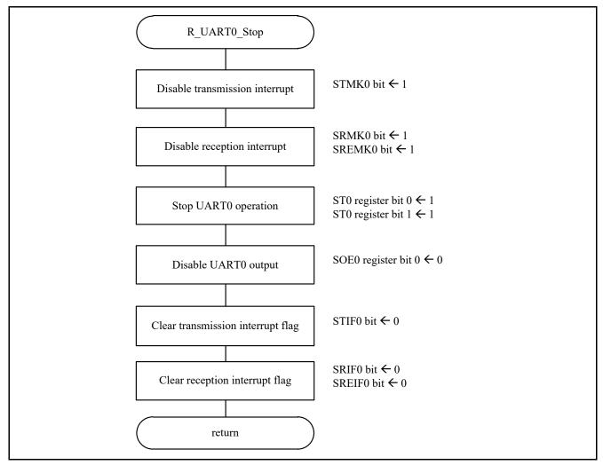
Figure 5.18 UART0 operation stop function
