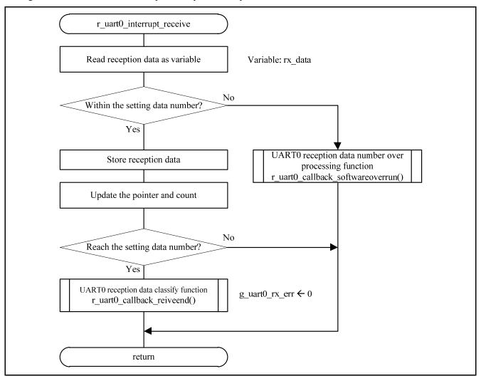
Figure 5.19 UART0 reception complete interrupt function
