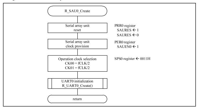
Figure 5.11 Serial array unit initialization function
