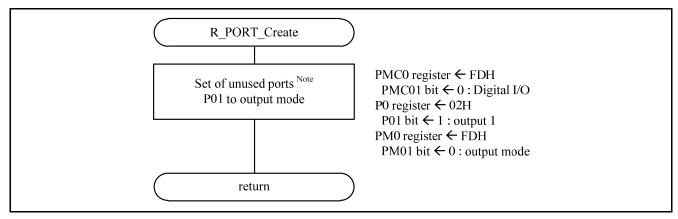
Figure 5.6 I/O Port Setup
