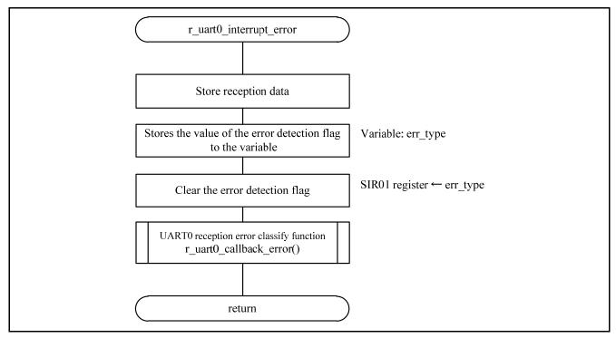
Figure 5.20 UART0 reception error interrupt function
