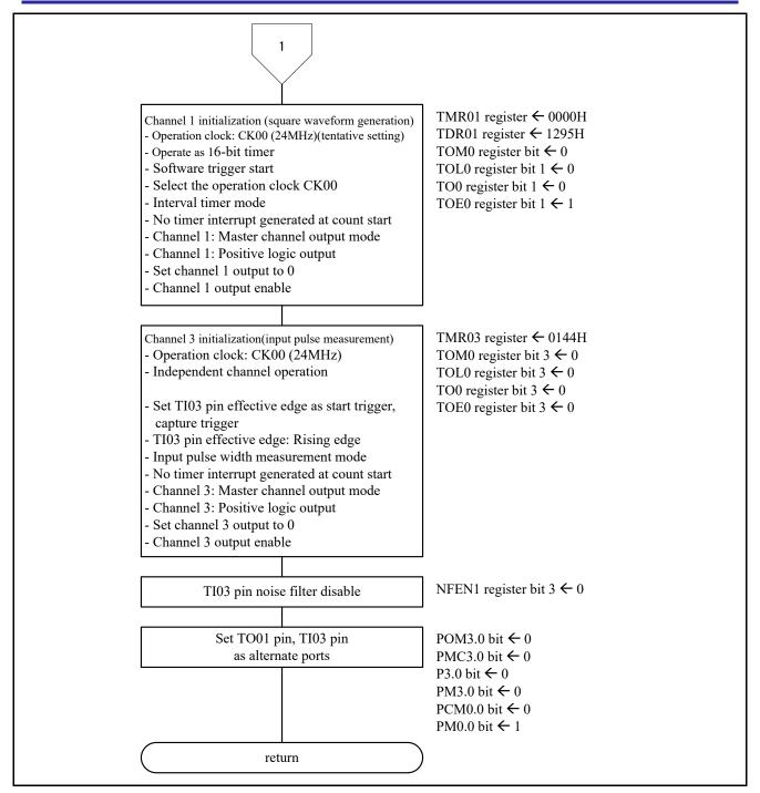
Figure 5.9 Timer array unit initialization(2/2)
