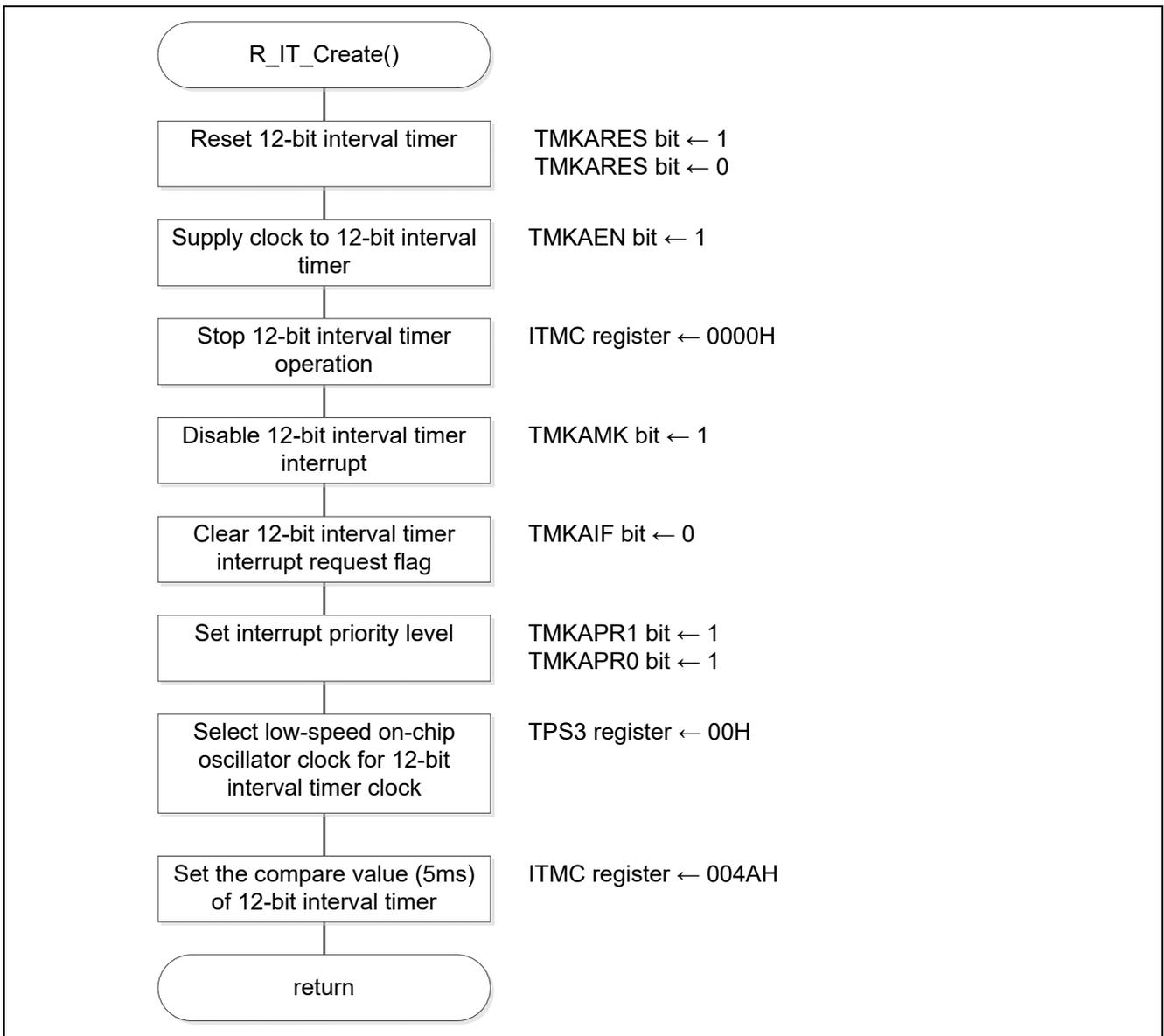
Figure 5.7 12-bit Interval Timer Setting
