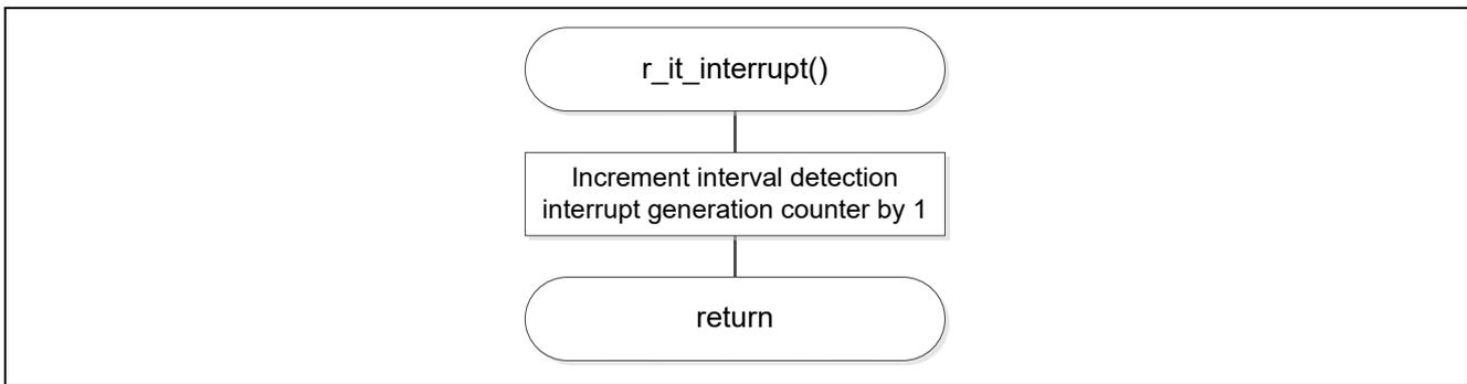
Figure 5.61 12-bit Interval Timer Interrupt Servicing
