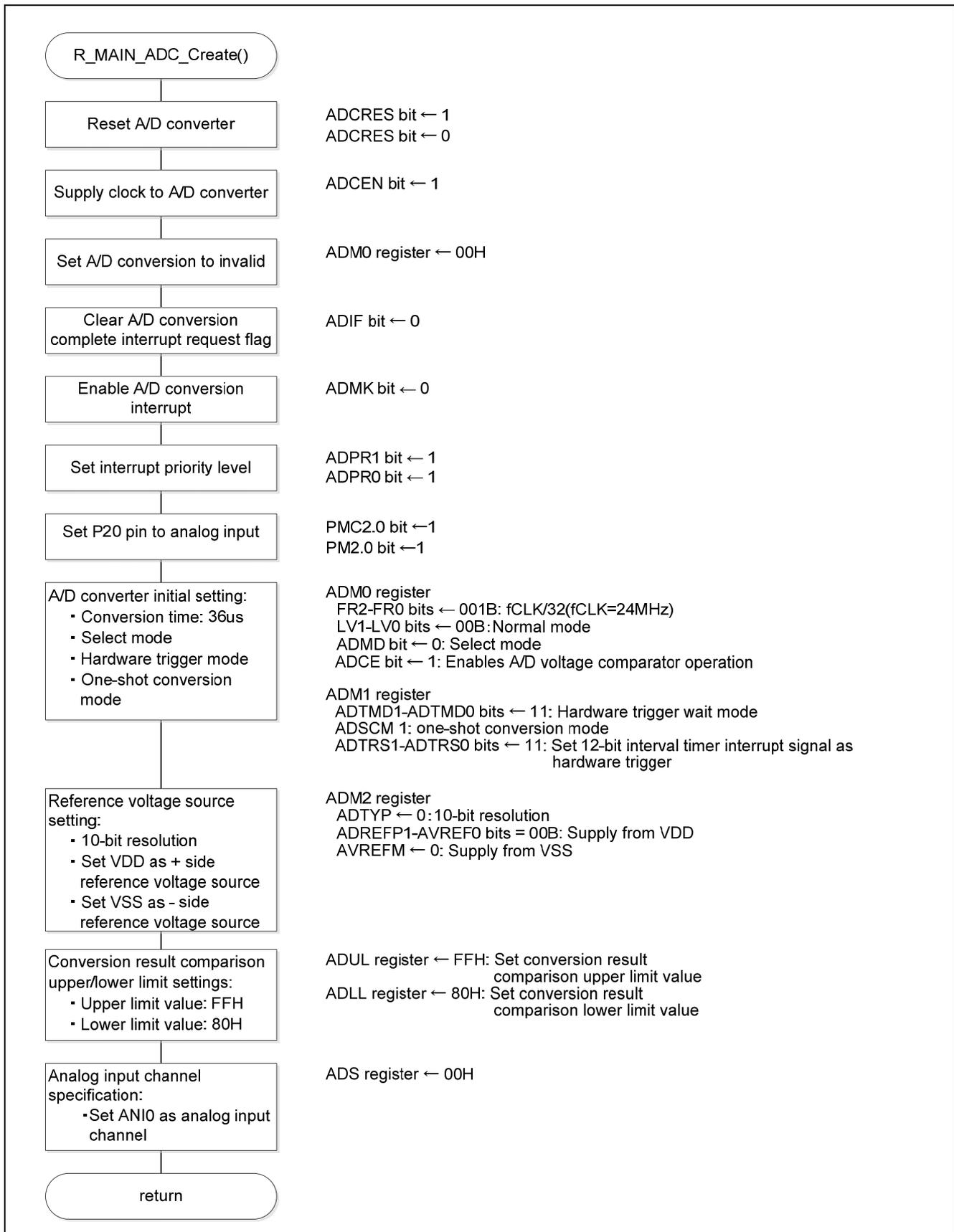
Figure 5.29 A/D Converter Initial Setting
