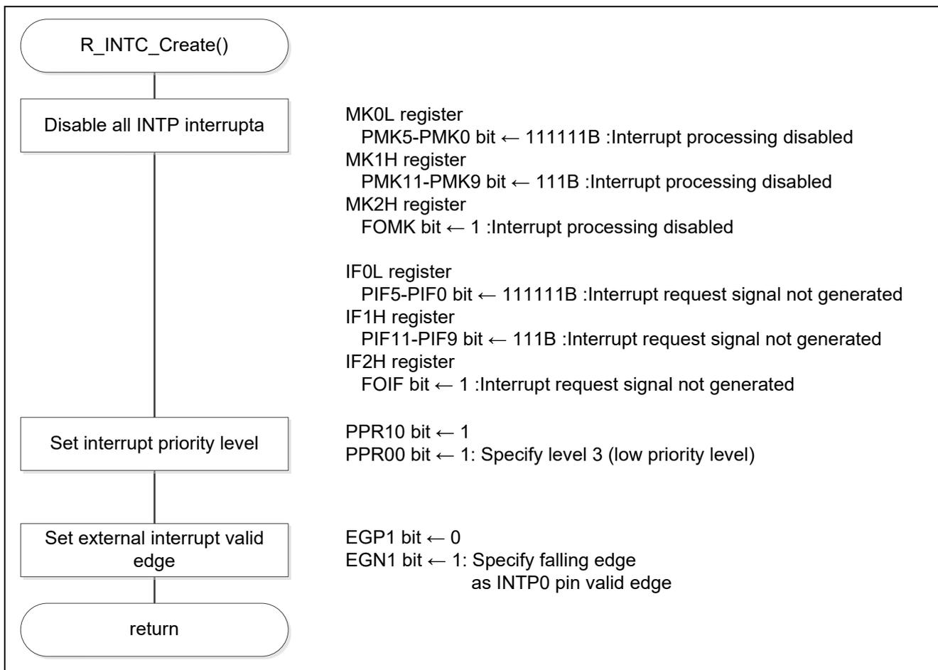
Figure 5.6 External Interrupt Setting
