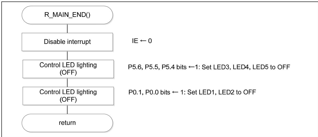
Figure 5.59 Status Transition End Processing
