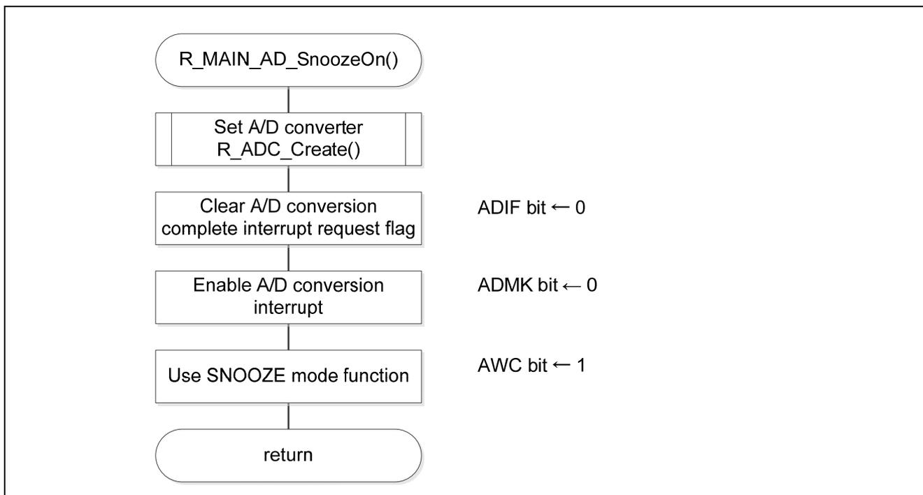
Figure 5.28 A/D Converter Setting
