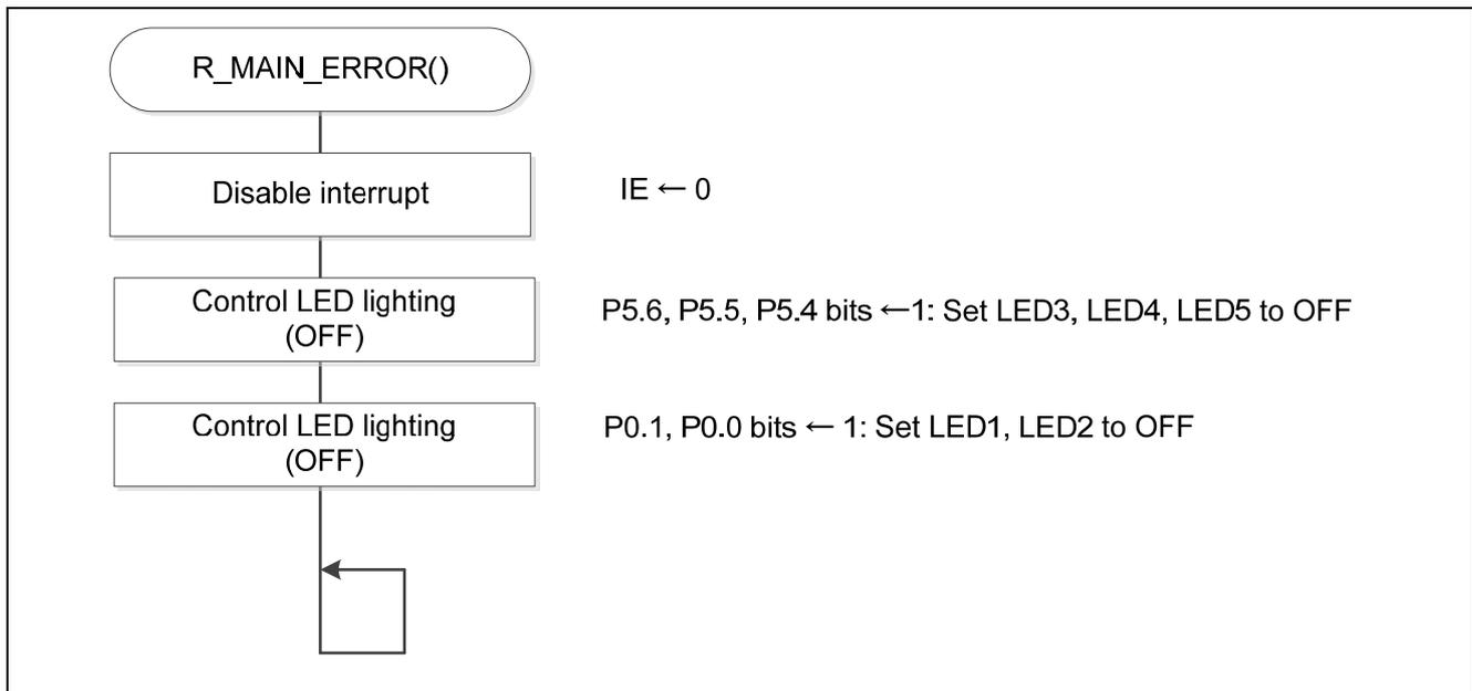
Figure 5.16 Error Processing of Status Transition
