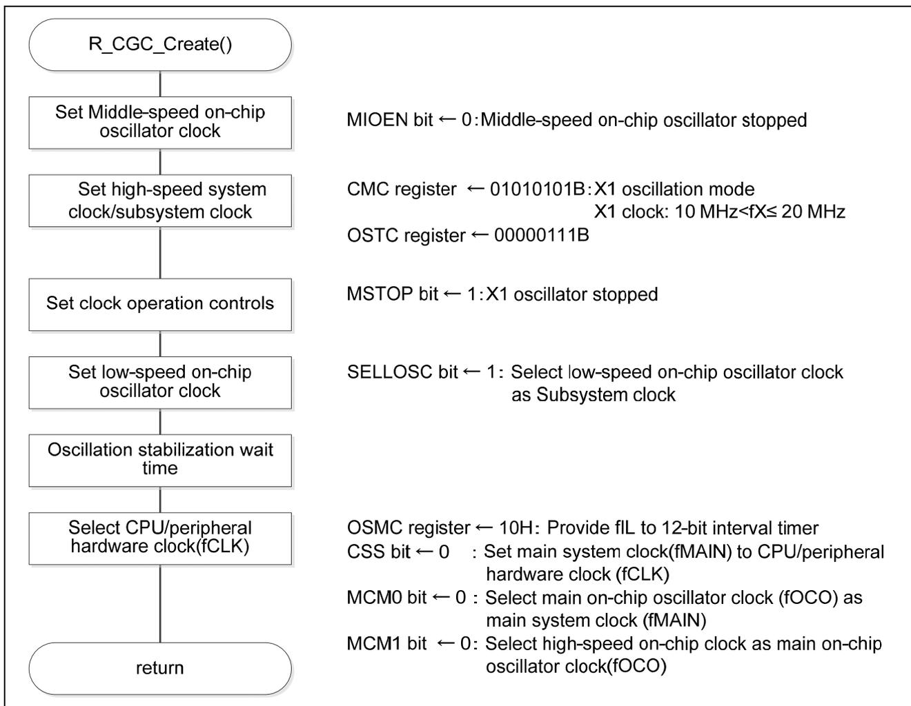
Figure 5.5 Clock Generator Setting
