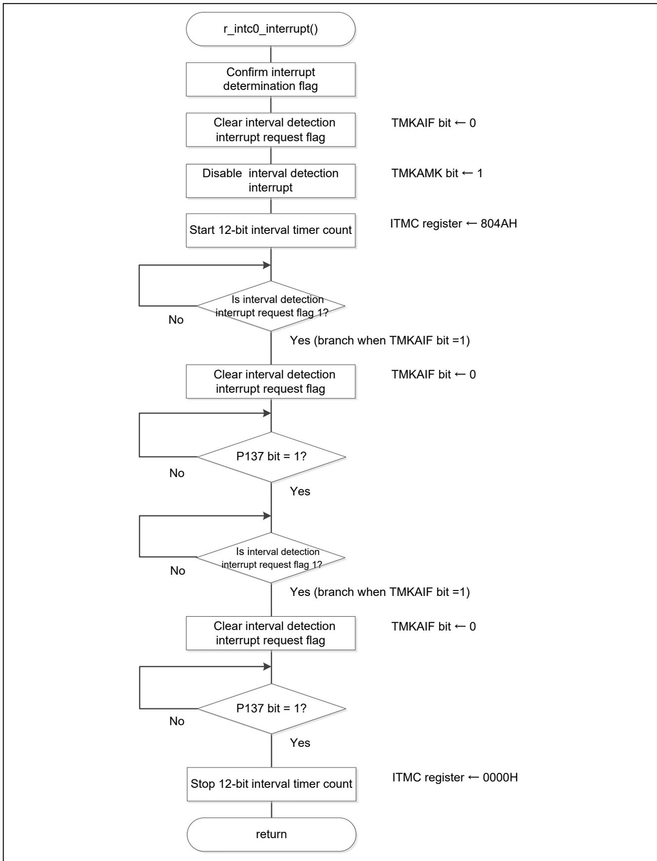
Figure 5.60 External Interrupt Servicing
