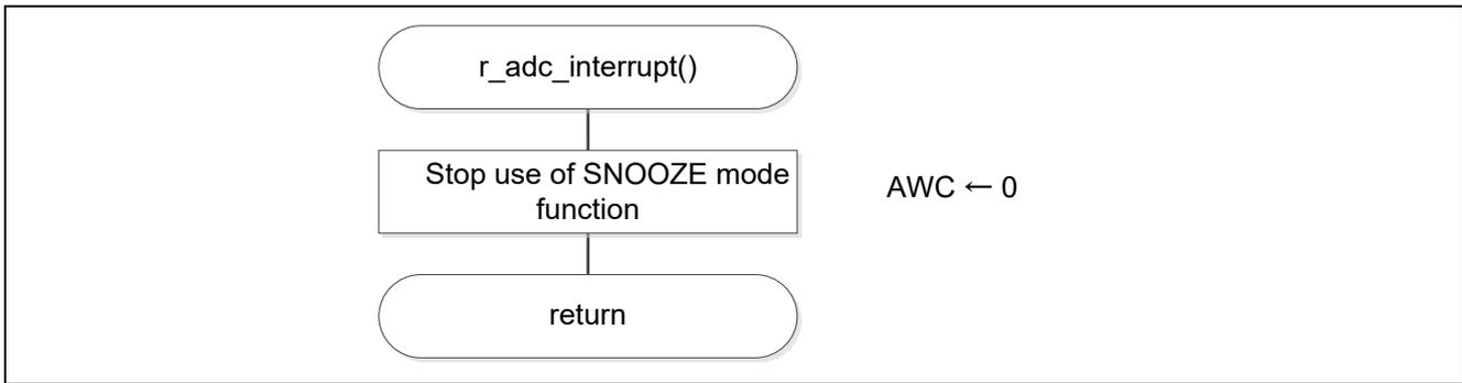
Figure 5.62 A/D Conversion Completion Interrupt Servicing
