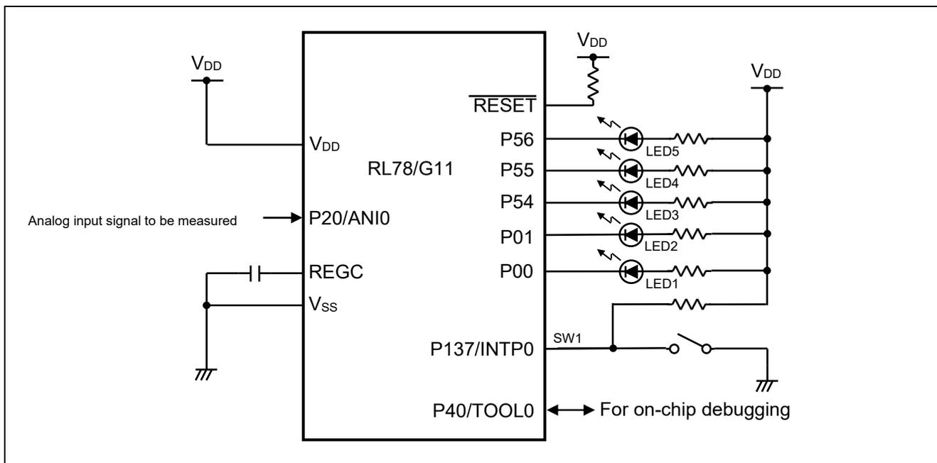
**Figure 4.1 Hardware Configuration**
