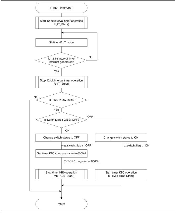
Figure 5.21 INTP1 External Interrupt Function
