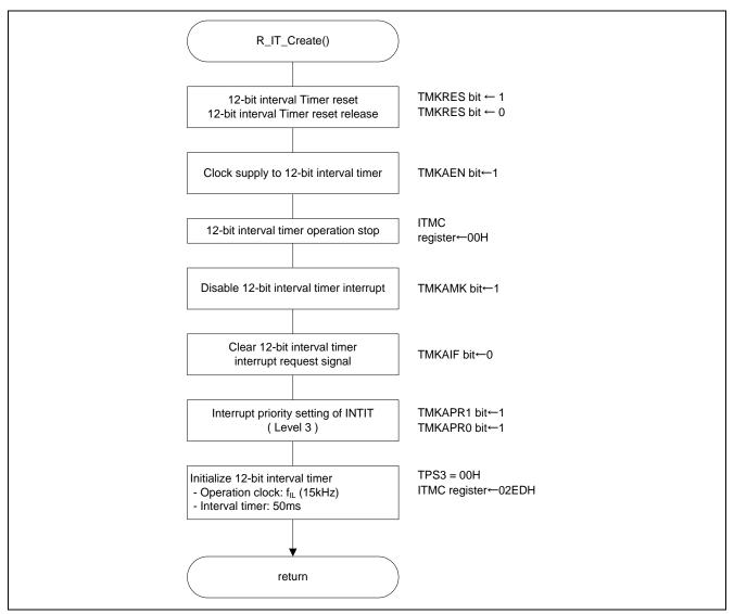
Figure 5.10 12-bit Interval Timer Initial Setting
