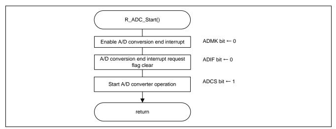
Figure 5.24 A/D Converter Operation Startup
