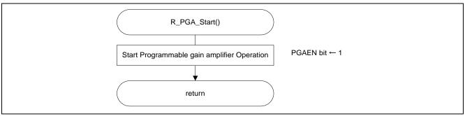
Figure 5.16 Programmable gain amplifier Operation Startup
