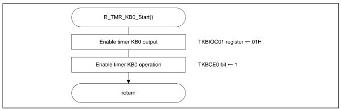
Figure 5.20 16-bit timer KB0 Operation Startup
