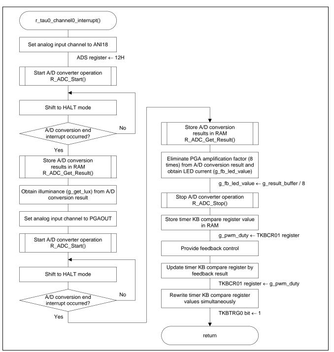
Figure 5.23 Timer Array Unit Interrupt Processing
