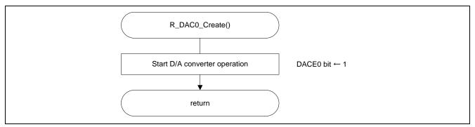
Figure 5.15 D/A converter Operation Startup
