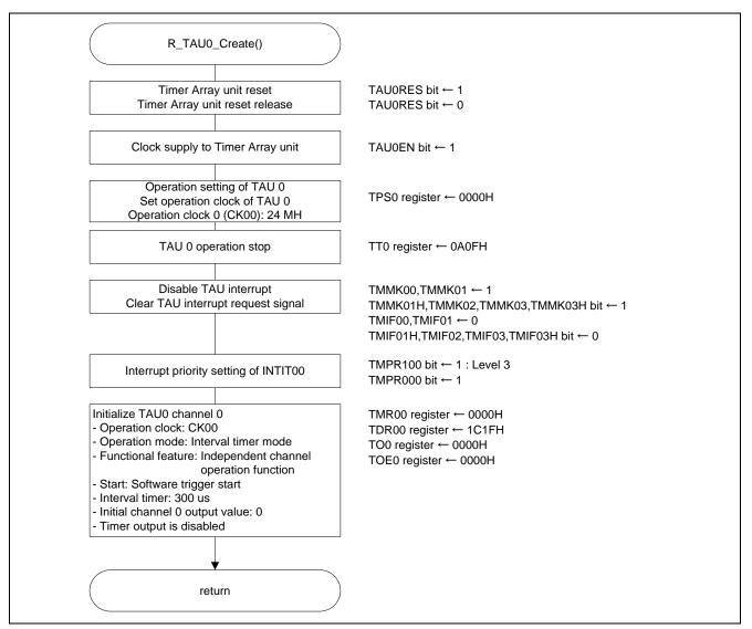
Figure 5.9 Timer Array Unit Initial Setting
