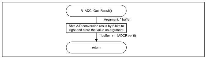
Figure 5.25 A/D Conversion Result Acquisition
