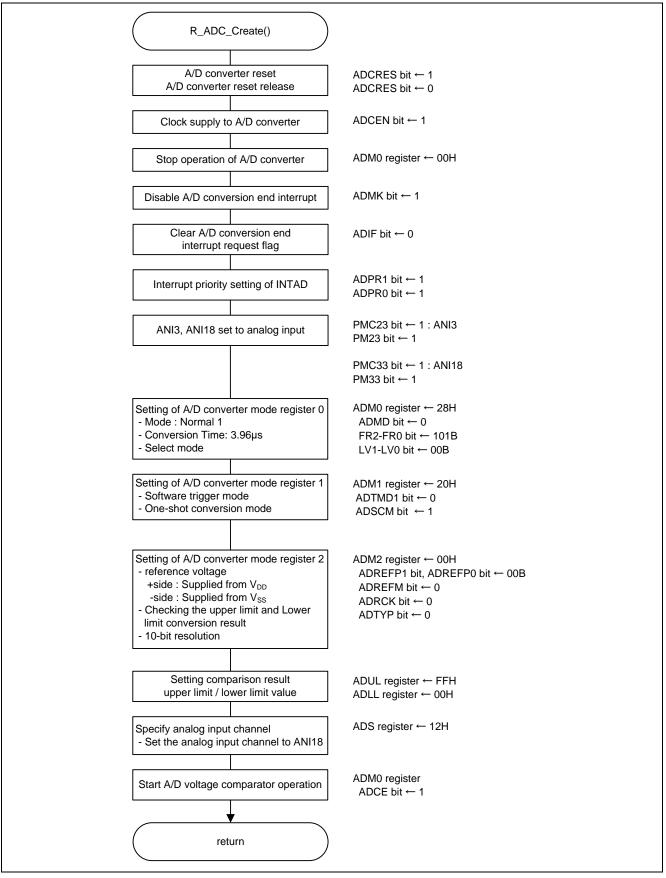
Figure 5.11 A/D Converter Initial Setting
