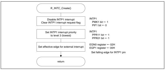
Figure 5.12 Initial Setting of External Interrupt
