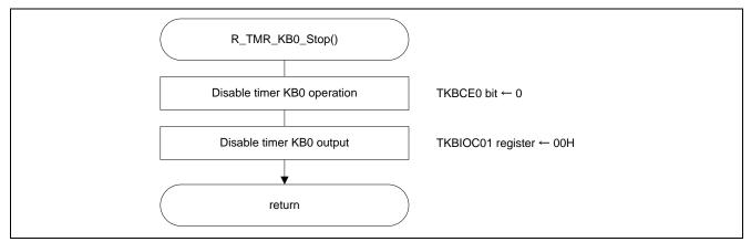
Figure 5.22 16-bit timer KB0 Operation Stop
