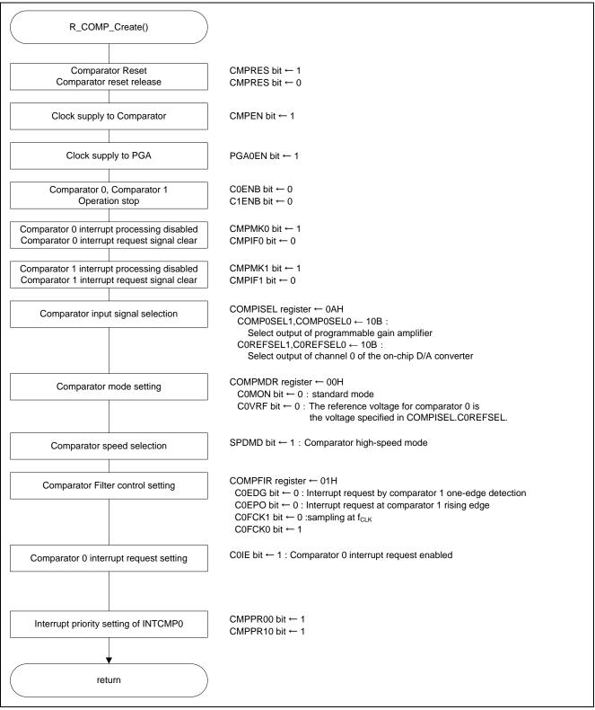
Figure 5.8 Comparator 0 Initial Setting
