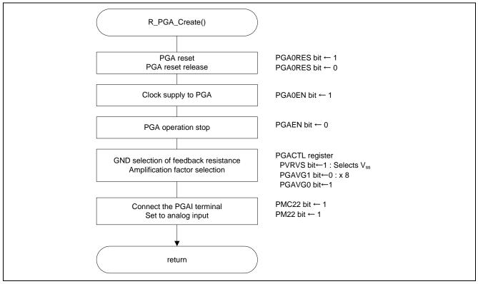
Figure 5.7 Programmable gain amplifier (PGA) Initial Setting
