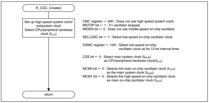
Figure 5.4 CPU Clock Setup
