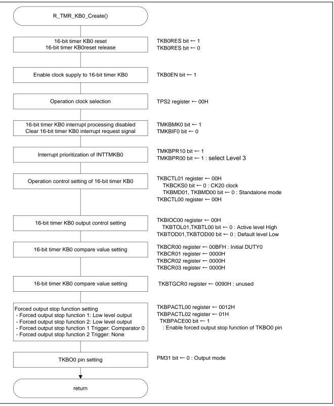
Figure 5.5 16-bit timer KB0 Initial Setting
