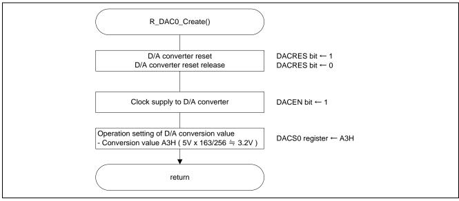
Figure 5.6 D/A Converter Initial Setting
