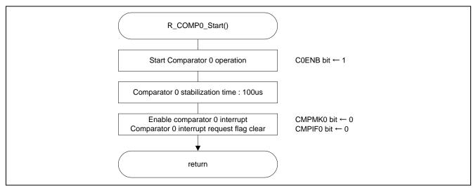
Figure 5.17 Comparator 0 Operation Startup
