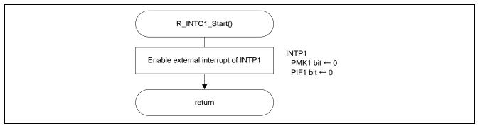
Figure 5.18 INTP1 External Interrupt Enabling Function
