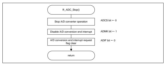
Figure 5.26 A/D Converter Operation Stop
