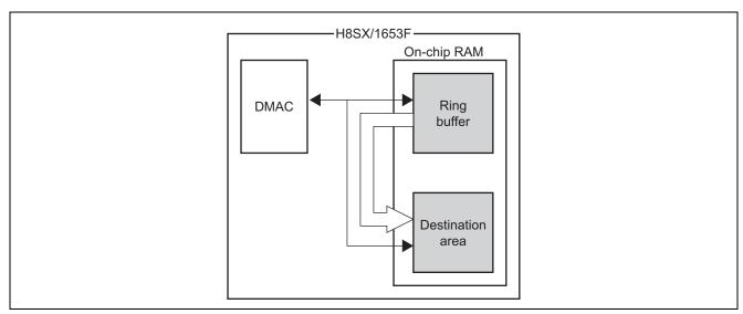
Figure 1 Ring Buffer Processing by DMAC Extended Repeat Transfer
