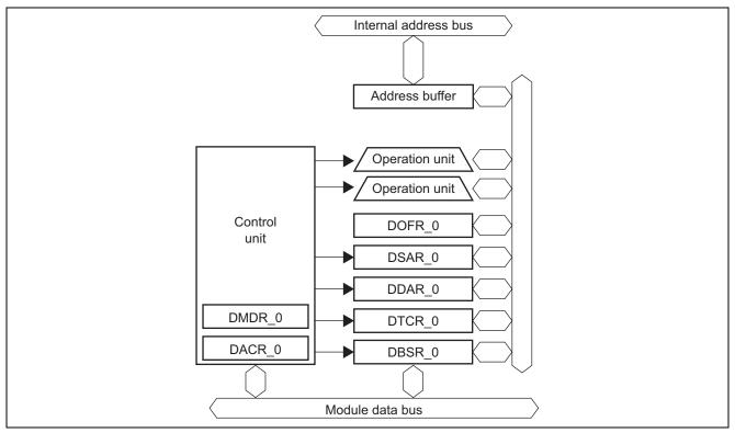
Figure 2 Block Diagram of DMAC
