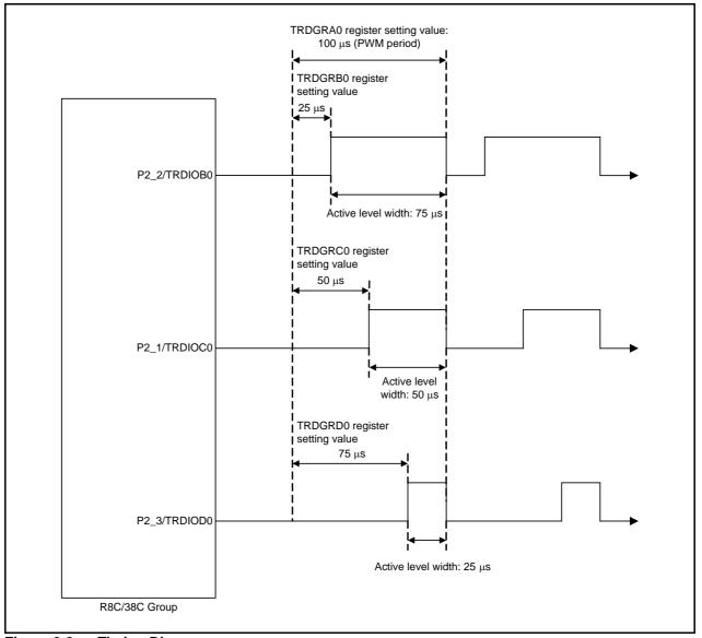
Figure 3.2 Timing Diagram
