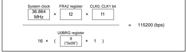
Figure 3.1 Bit Rate Setting Values
