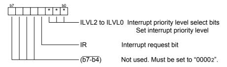
(\*) Use "OR" instruction so that the interrupt request bit is not changed when setting the interrupt priority level.
