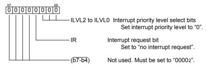
(9) G1IE0 register (interrupt enabled register reset)
