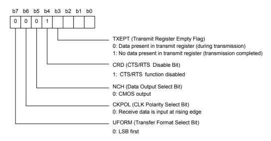
• Set up the U0C1 register (UART0 transmit/receive control register 1)
