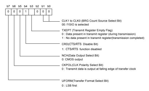
• Set up the U0C1 register (UART0 transmit/receive control register 1)
