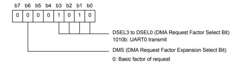
• Set up the DM0CON register (DMA0 control register)
