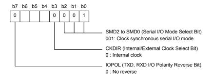
• Set up the U0C0 register (UART0 transmit/receive control register 0)
