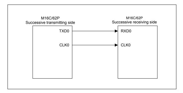
Figure 1. Example Connection for Successive Transmission/Reception
