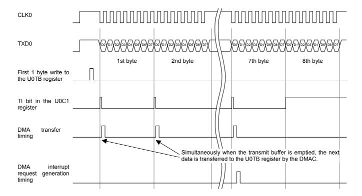
Figure 2. Successive Transmission/reception Timing
