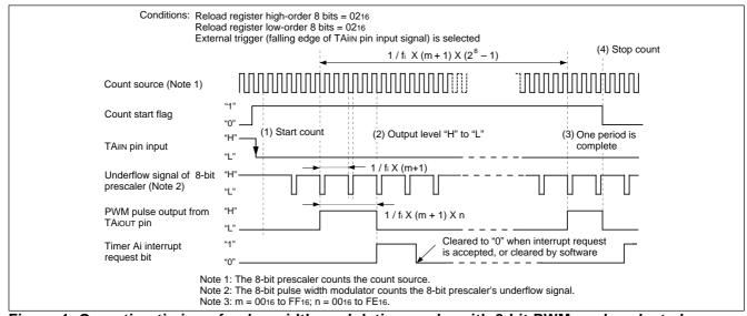
Figure 1. Operation timing of pulse width modulation mode, with 8-bit PWM mode selected
