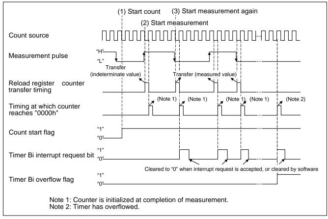
Figure 1. Operation Timing of Pulse Width Measurement Mode
