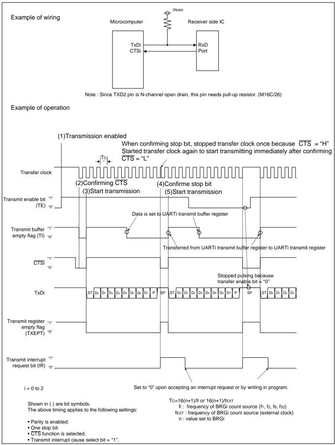
Figure 1. Operation Timing of Transmission in Clock-asynchronous Serial I/O Mode
