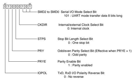
(2) Setting UART2 transmit/receive control register 0
