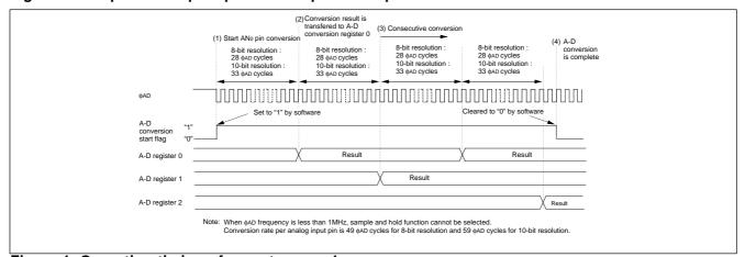
Figure 1. Operation timing of repeat sweep 1
