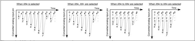
Figure 1. ANi pin's sweep sequence in repeat sweep mode
