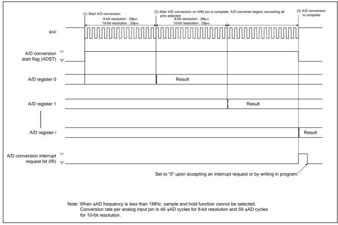
Figure 1. Operation Timing of Single Sweep Mode
