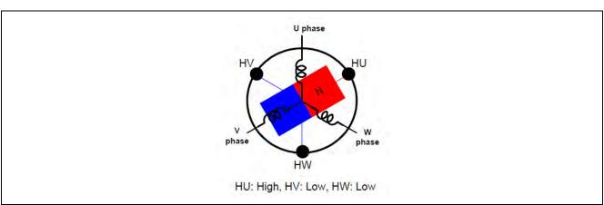
Figure 3-1 Example of hall sensor (HU, HV, HW) position and position signal
