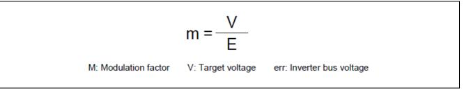
This modulation factor is reflected in the setting value of resistor that determines the PWM duty.
