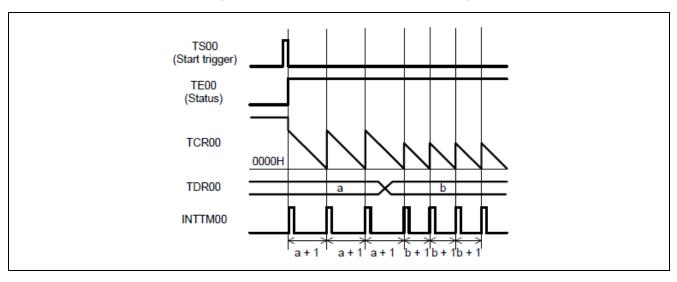
Figure 4-2 Example of basic timings of interval timer (Example of Channel 0)
