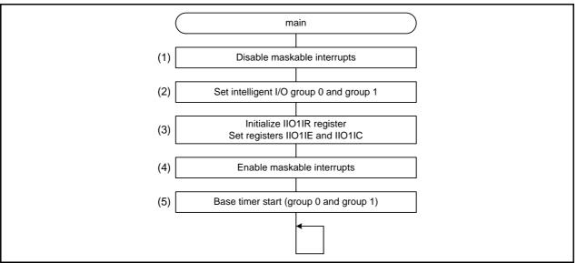
Figure 4.3 main Function Flowchart
