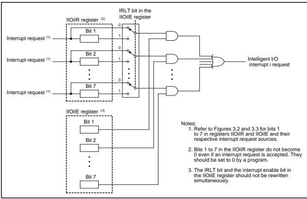
Figure 3.1 Intelligent I/O Interrupt Block Diagram (i = 0 to 11)
