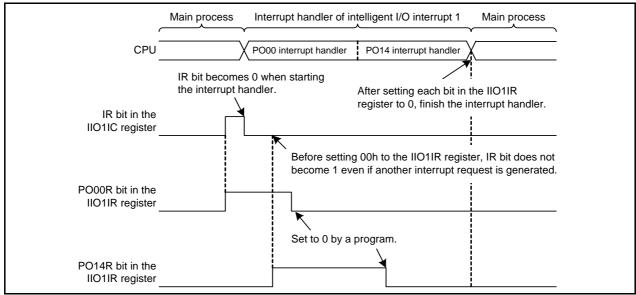
Figure 4.1 Operation Example of Intelligent I/O Interrupt 1
