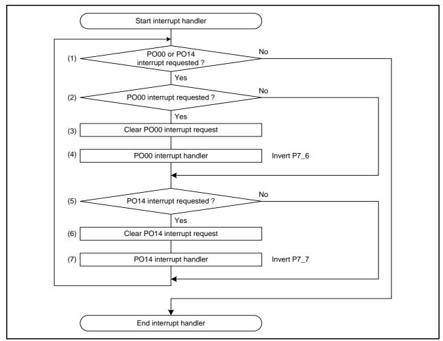
Figure 4.4 Function Flowchart of Intelligent I/O Interrupt 1
