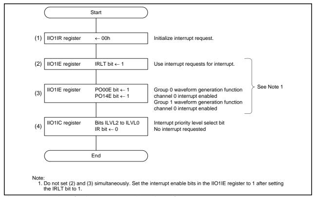
Figure 4.2 Register Setting Procedure of Intelligent I/O Interrupt 1
