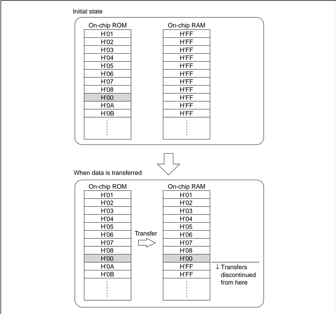
Figure 2 Example of MOVSD Block Transfer Instruction Operation
