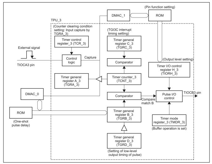
Figure 2 Block Diagram of One-Shot Pulse Output
