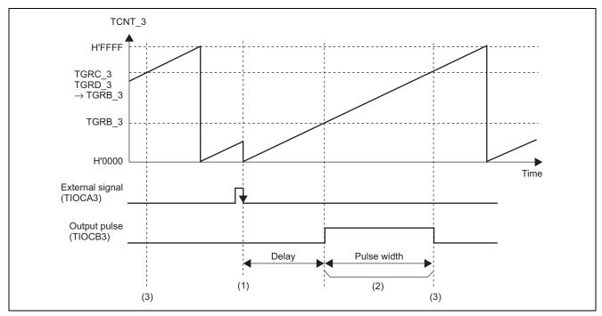
Figure 3 Operation of One-Shot Pulse Output
