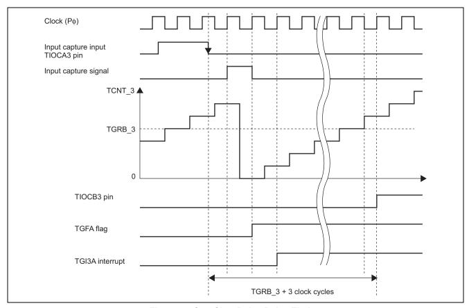
Figure 4 One-Shot Pulse Delay Timing
