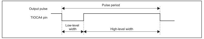
Figure 1 Example of Long-Period Pulse Output
