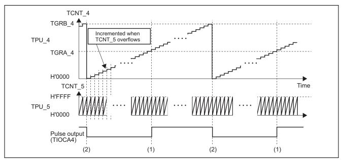
Figure 3 Operation of Long-Period Pulse Output
