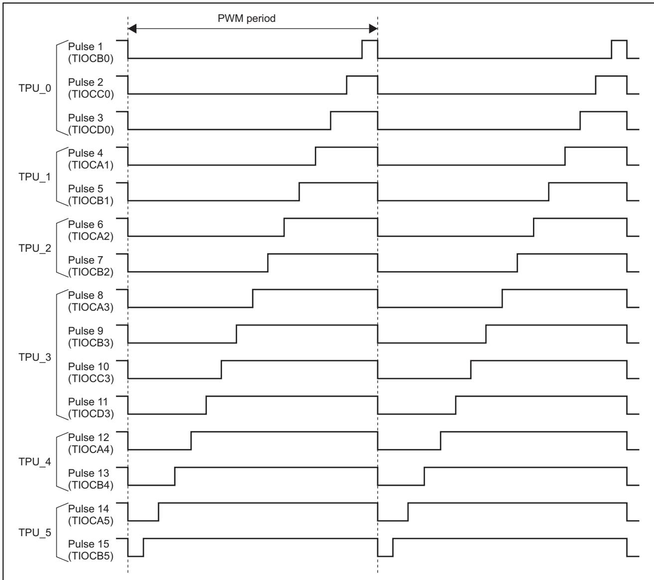
**Figure 1 Example of 15-Phase PWM Output**
