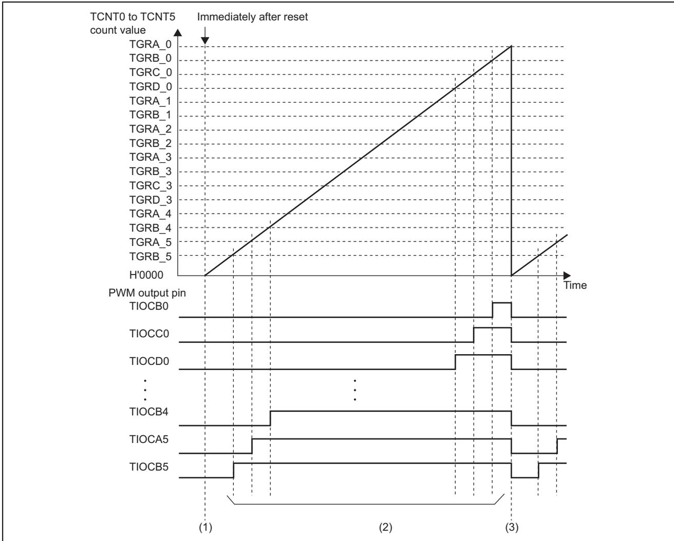
Figure 3 Operation of 15-Phase PWM Output
