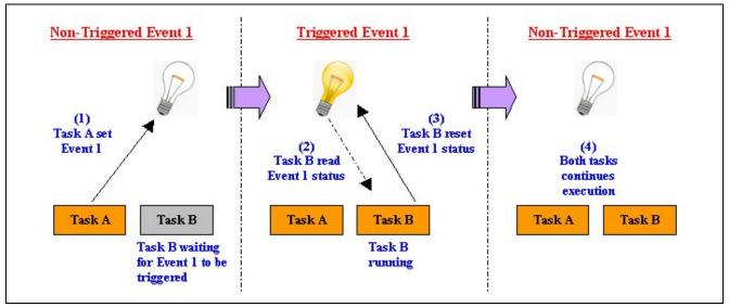
Figure 12 Working Principle of Event Objects
