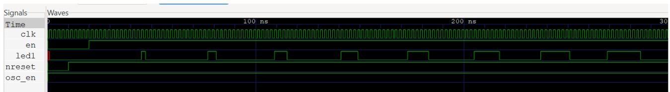
Figure 2: Single channel Breathing Functional Waveform
