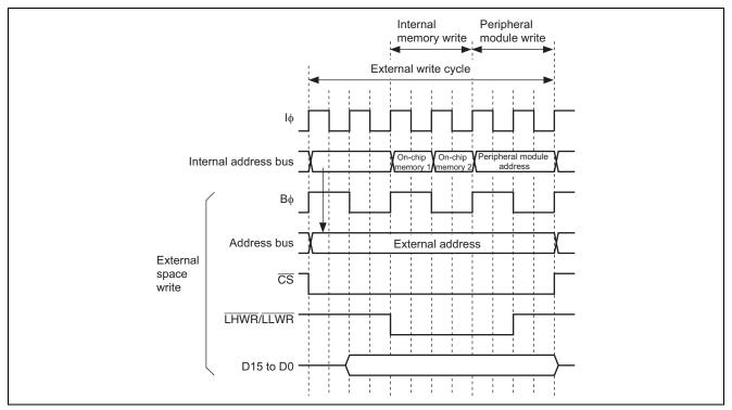
Figure 2 Example of Timing when the External-Write-Data Buffer is in Use (WDBE = 1)
