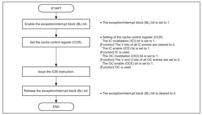
Figure 6 Procedure for Cache Settings
