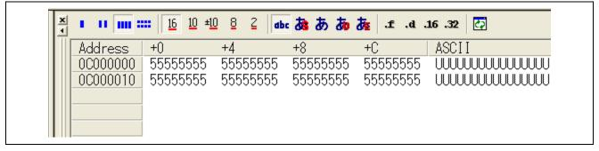
Figure 11 Memory Dump from Access to the Cacheable P0 Area
