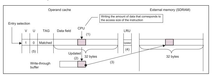
Figure 1 Write-Through Mode (Cache Hit)
