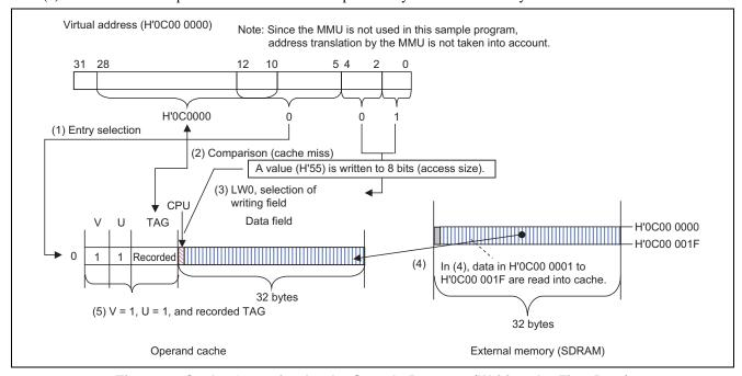
Figure 8 Cache Operation by the Sample Program (Writing the First Byte)
