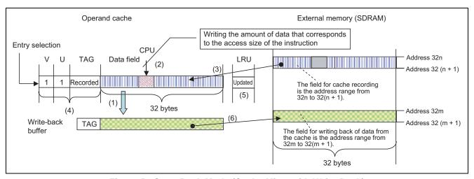
Figure 5 Copy-Back Mode (Cache Miss, with Write-Back)
