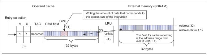
Figure 4 Copy-Back Mode (Cache Miss, without Write-Back)
