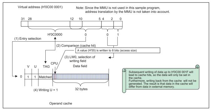
Figure 9 Cache Operation by the Sample Program (Writing the Second Byte)
