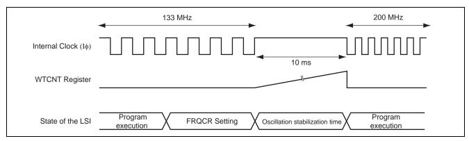
Figure 4 Operation Timing of Sample Program
