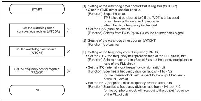
Figure 3 Example Flow for Settings to Change the Operating Frequency
