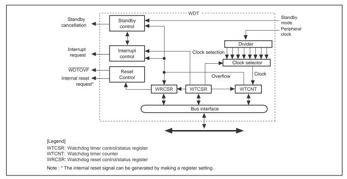
Figure 2 Block Diagram of the WDT
