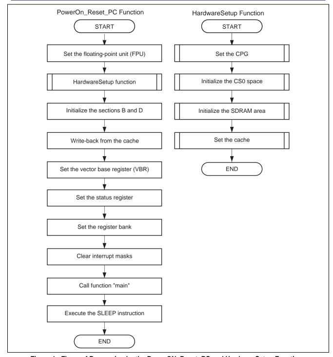
Figure 1 Flows of Processing by the PowerON\_Reset\_PC and HardwareSetup Functions
