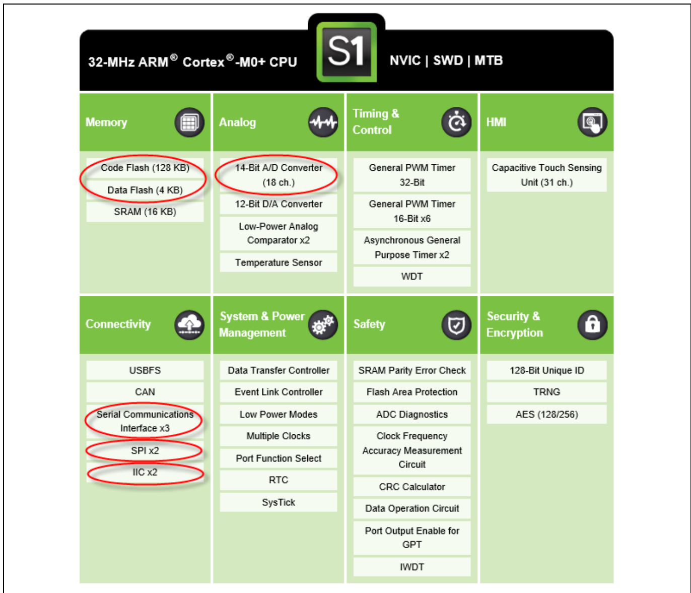
Figure 1. S1 peripherals used by the OoB
