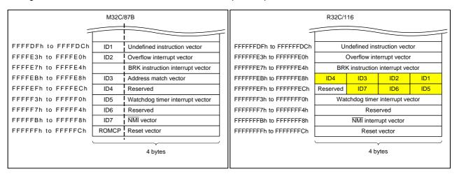
Figure 4.2 Comparison Diagram: Addresses for ID Code Stored
