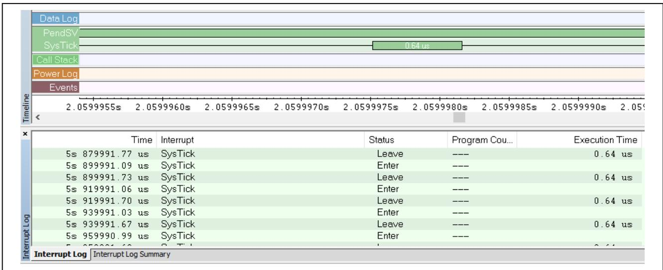
**Figure 28 SysTick timing**
