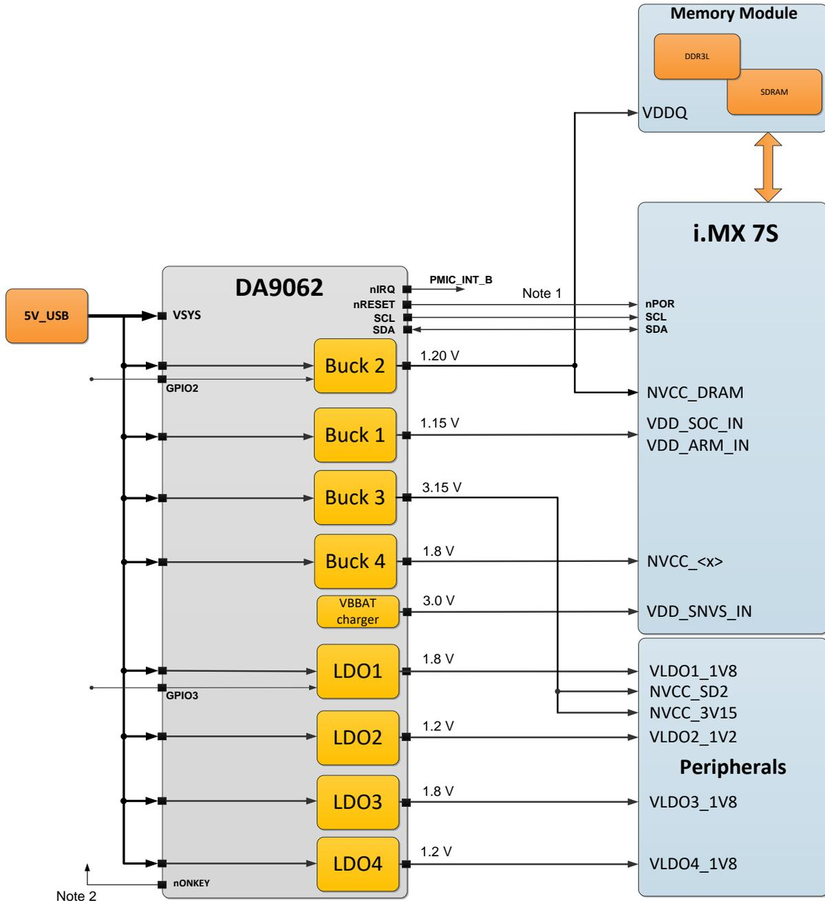
Figure 3: DA9062 Connections to WaRP7 Demo Board
