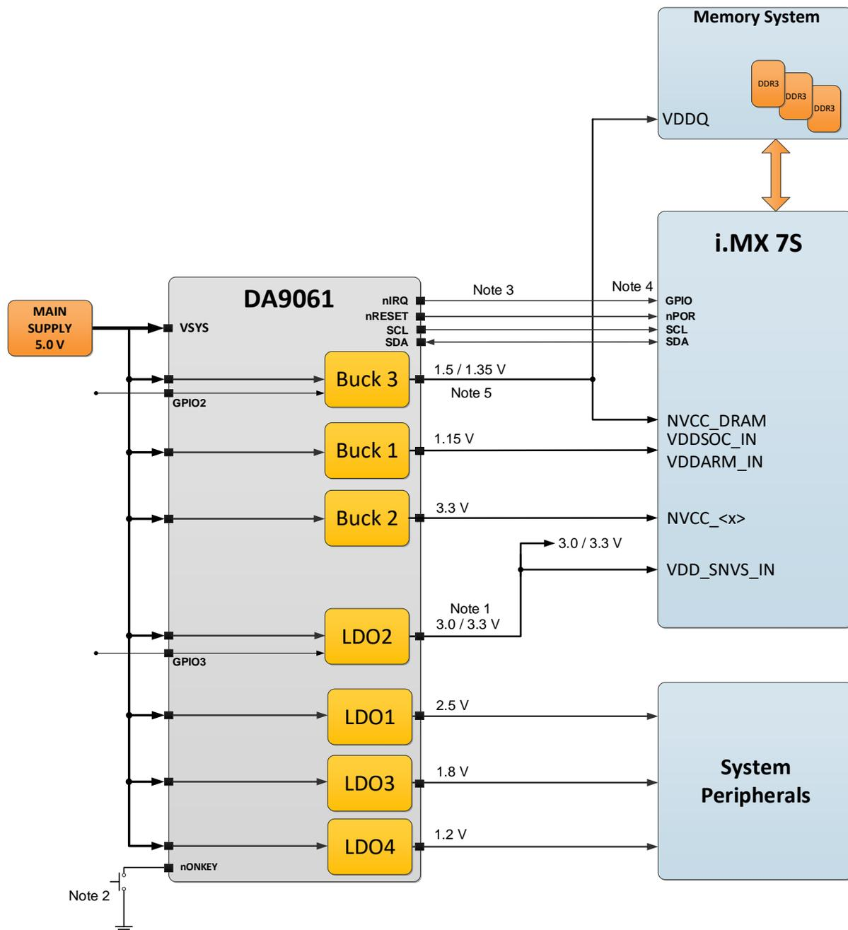
Figure 1: DA9061 Connections to i.MX 7Solo
