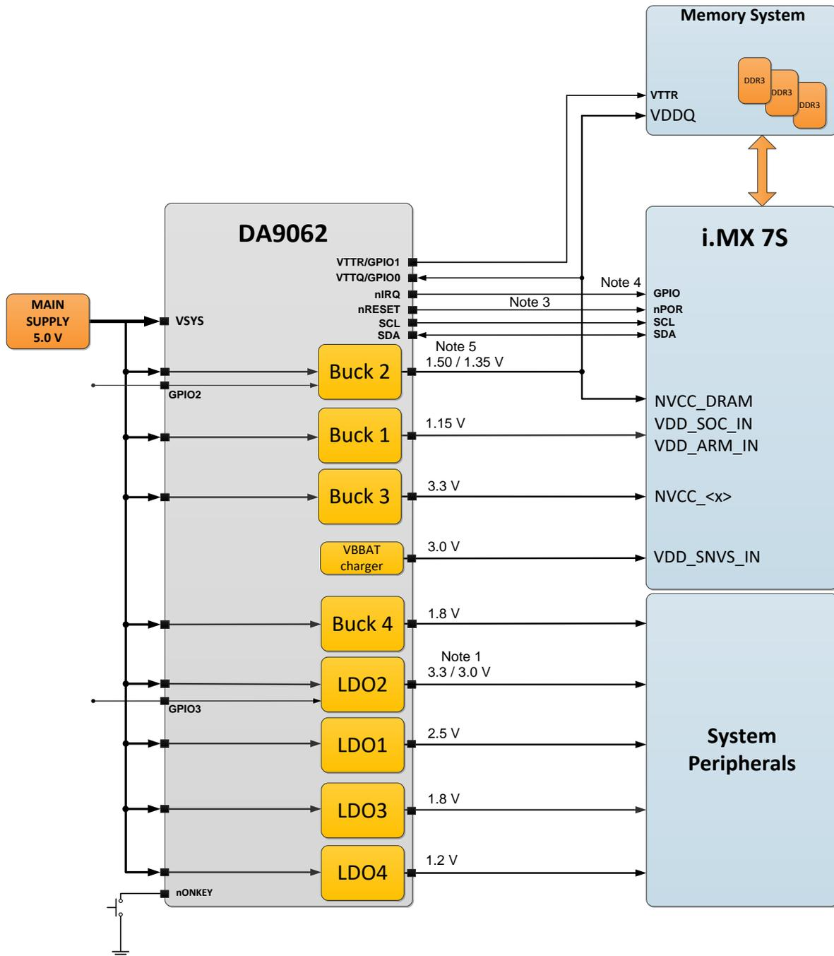
**Figure 2: DA9062 Connections to i.MX 7S**
