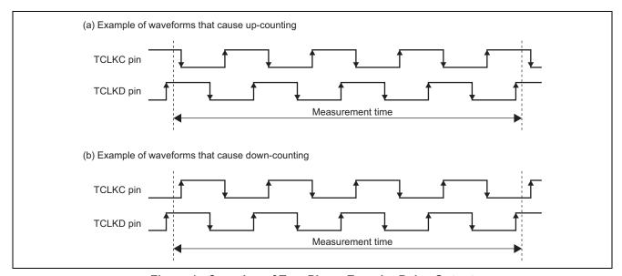
Figure 1 Counting of Two-Phase Encoder Pulse Output
