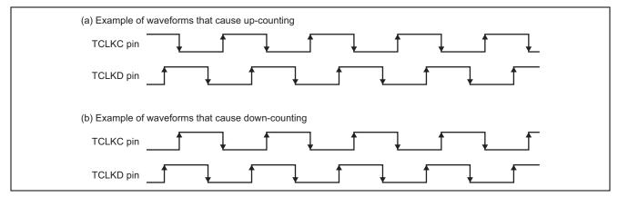
Figure 3 Example of Phase Counting Mode 1 Operation
