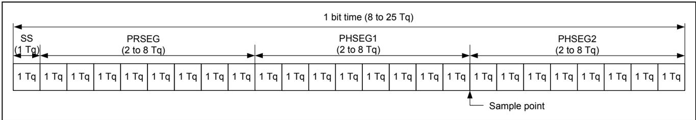
**Figure 4 Bit Configuration**
