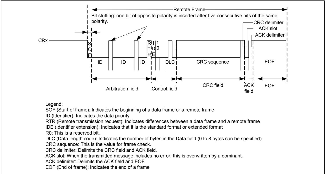
**Figure 5 CAN Reception Waveform**
