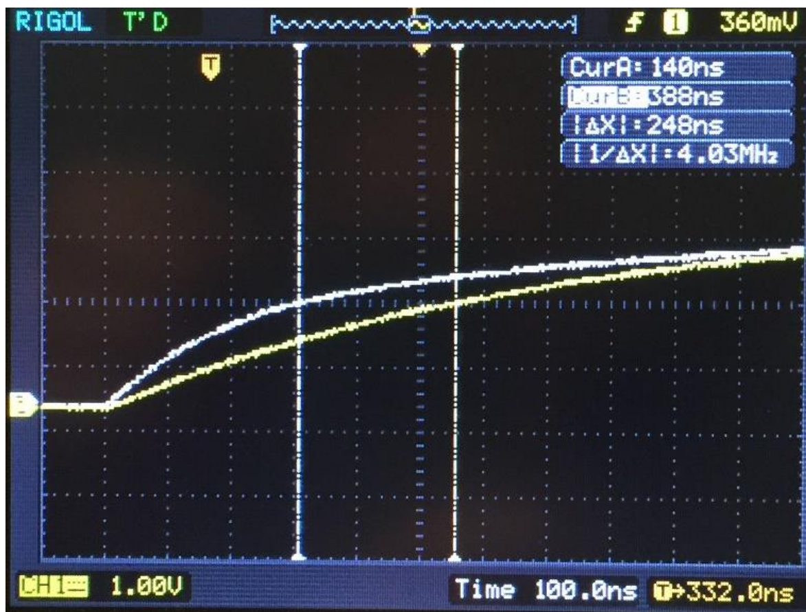
Figure 2: Oscilloscope Capture Showing the Difference in Risetime
