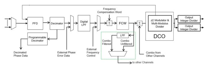
Figure 1. Block Diagram of One Channel of ClockMatrix
