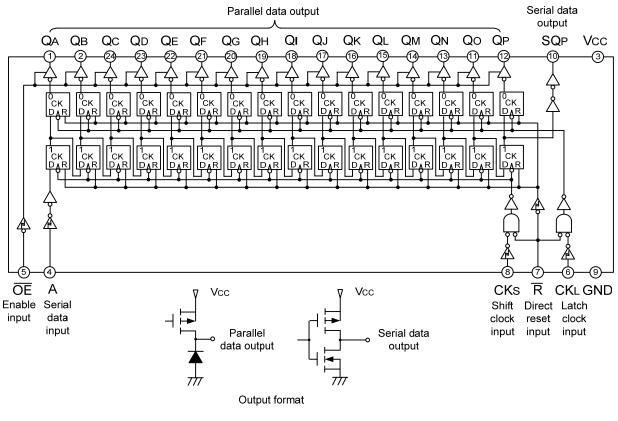
Figure 3.2 M66310P/FP Structure Diagram
