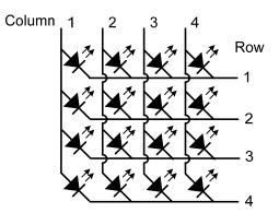
Figure 3.1 A Sample Structure of a Unicolor 4x4 LED Matrix
