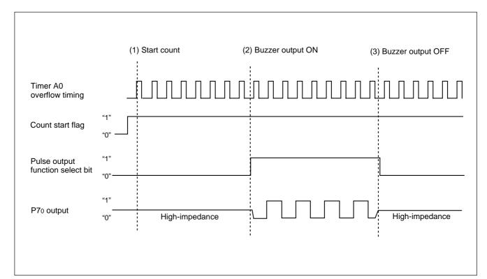
Figure 1. Operation timing of buzzer output
