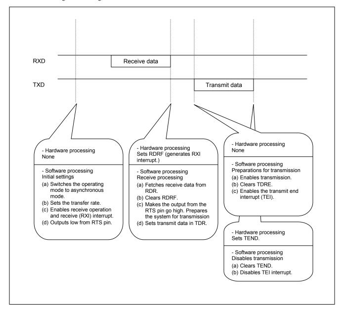
Figure 4 Description of Operation of Asynchronous SCI
