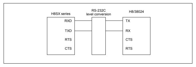
Figure 1 Block Diagram of the Asynchronous SCI Using the H8SX Series
