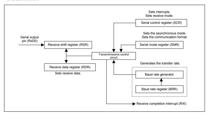
Figure 3 Block Diagram of SCI Reception
