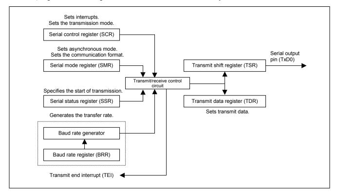
Figure 2 Block Diagram of SCI Transmission
