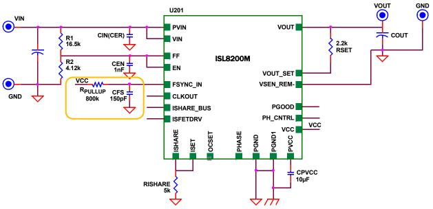
FIGURE 2. APPLICATIONS CIRCUIT FOR REDUCING FSW
