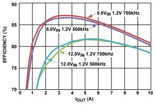
FIGURE 3. EFFICIENCY WITH V<sub>OUT</sub> = 1.2 AT V<sub>IN</sub> = 5V AND 12V AND F<sub>SW</sub> = 700Hz AND 500kHz
