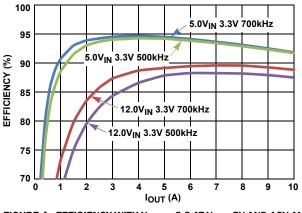
FIGURE 4. EFFICIENCY WITH V\_{OUT} = 3.3 AT V\_{IN} = 5V AND 12V AND F\_{SW} = 700Hz AND 500kHz
