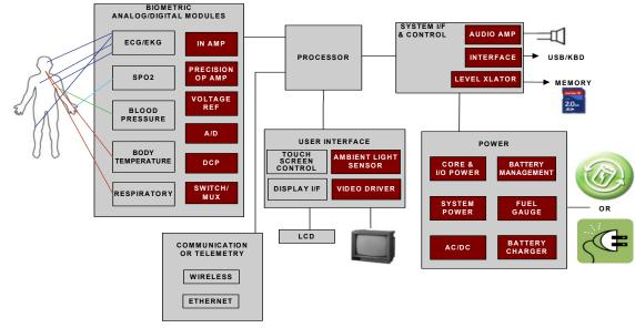
FIGURE 1. BLOCK DIAGRAM OF A PATIENT MONITOR
