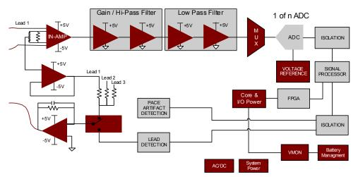
FIGURE 3. BLOCK DIAGRAM OF AN ECG SYSTEM
