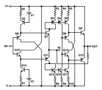
FIGURE 3. CURRENT FEEDBACK AMPLIFIER SIMPLIFIED SCHEMATIC
