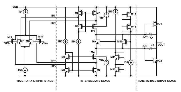
FIGURE 4. SIMPLIFIED SCHEMATIC OF A CMOS RAIL-TO-RAIL I/O AMPLIFIER
