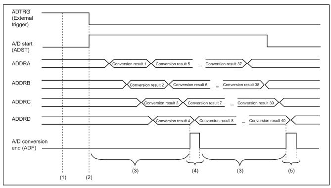
Figure 3 Principles of A/D Conversion in Scan Mode
