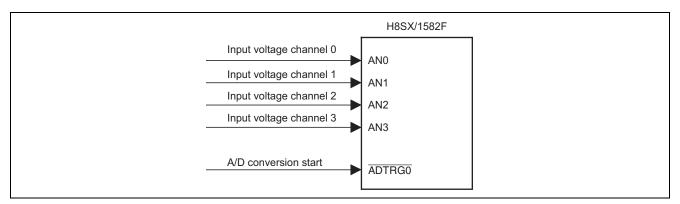
Figure 1 A/D Conversion in Scan Mode
