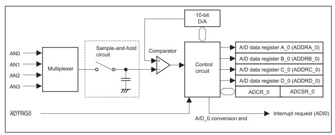
Figure 2 Block Diagram of A/D Converter
