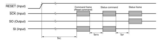
(d) Chip Erase command/Block Erase command/ Block Blank Check command/Oscillating Frequency Set command
