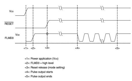
Figure 2-6. Setting Flash Memory Programming Mode and Selecting Communication Mode
