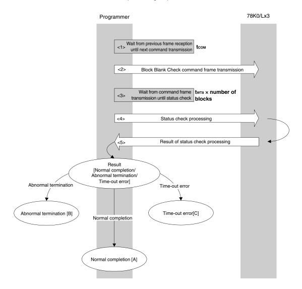
Block Blank Check command processing sequence
