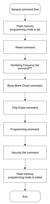
Figure 3-1. General Command Execution Flow at Flash Memory Rewriting
