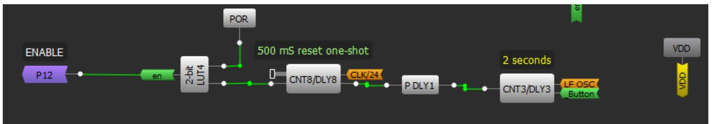
Figure 6. 5 second triggered 500ms Reset One-Shot
