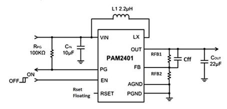
Figure 3. A Typical Boost Converter
