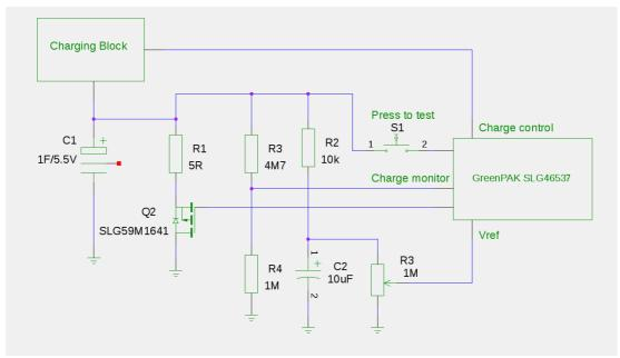
Figure 4. ESR Test - Schematic
