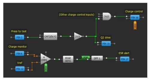
Figure 5. ESR Test - GreenPAK Designer Diagram
