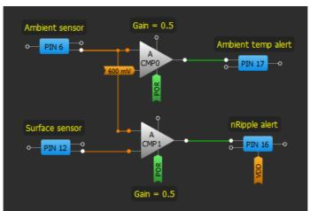
Figure 7. Temperature/Ripple Monitoring – GreenPAK Designer Diagram
