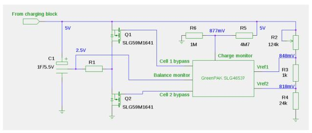
Figure 1. Cell Balancing - Schematic
