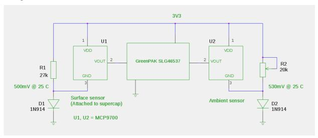
Figure 6. Temperature/Ripple Monitoring - Schematic
