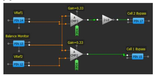
Figure 2. Cell Balancing – GreenPAK Designer Diagram
